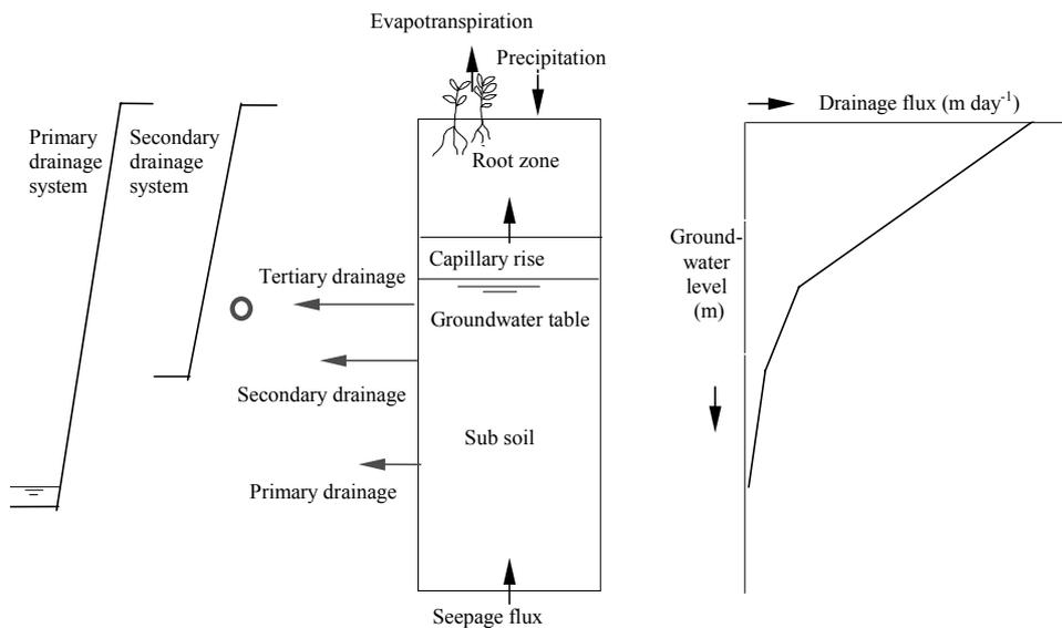
**Figure 1: Plot schematisation and drainage relations within MOZART**
