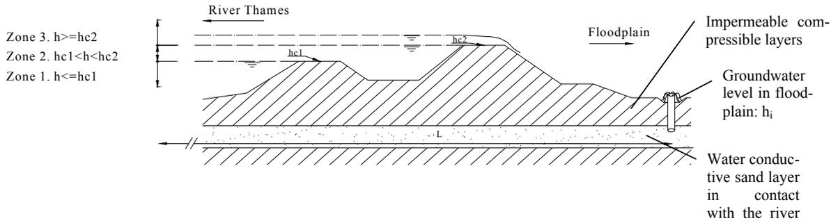
Figure 2. 'Double crested' earth embankments and the definition of three zones of water levels
