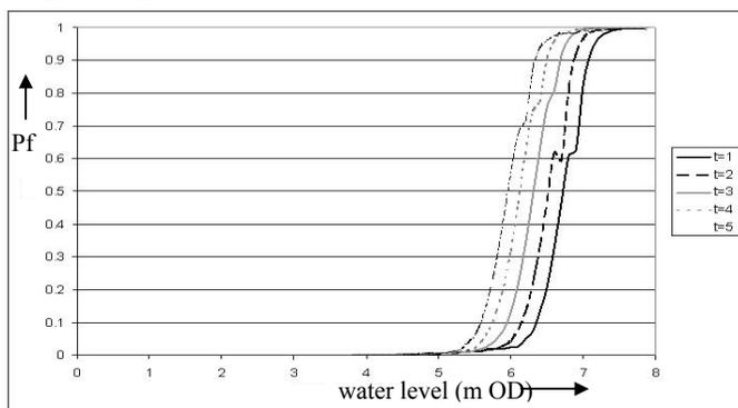
Figure 5. Time dependent probabilities of failure given different water levels, and given a significant wave height  $H_s = 1.0\text{m}$ , and a peak wave period,  $T_p = 8$ . The time  $t$  is in years.
