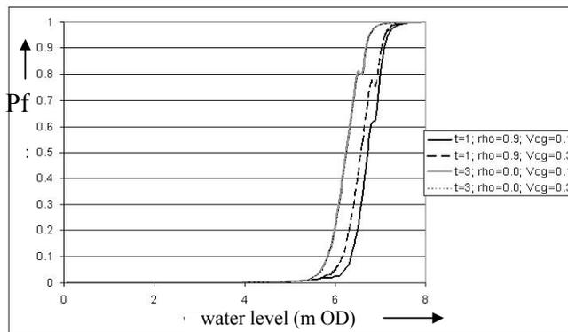
Figure 7. The change in overall probability of failure with a changing variation coefficient of the vegetation deterioration for  $\rho = 0.9$  and  $\rho = 0$ , between the crest level and vegetation deterioration processes. Different times are chosen to enhance the clarity of the figure.
