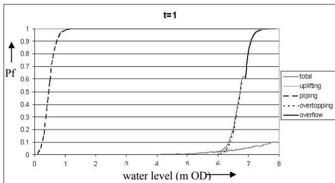
Figure 6. Contribution of the different failure modes in the different zones. Failure modes considered to be independent
