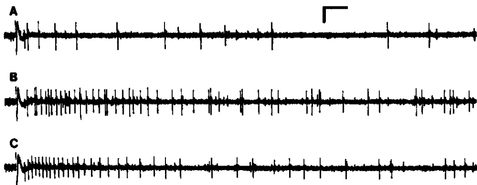
Fig. 2. Representative responses of one tarsal taste hair to (A) 0.05 NaCl, (B) eggwash (1000 ee/ml) and (C) 0.02 M glucotropaeolin. Stimuli B and C were dissolved in 0.05 M NaCl. Calibration: 0.8 mV; 50 ms.
