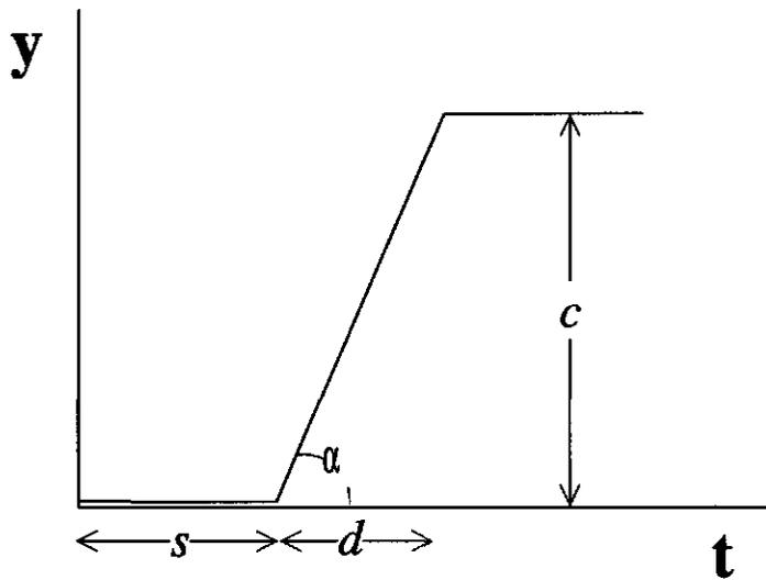
Fig. 3.1 The piecewise linear regression model for emergence ( $y$ ) against time after planting ( $t$ ). Parameter  $s$  is the time until start of emergence, parameter  $d$  is the duration of emergence, parameter  $c$  is the final level of emergence and parameter  $b (= \tan(\alpha) = c/d)$  is the rate of emergence.
