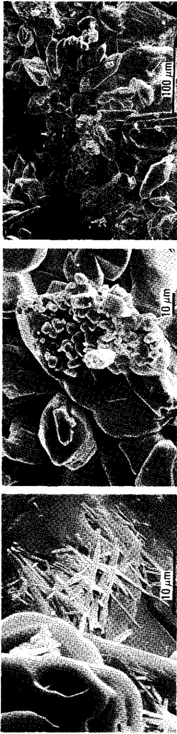
Fig.7.3 a.Thenardite crystals with bloedite and eugsterite. b.Enlargement of the bloedite crystals. c. Enlargement of eugsterite.
