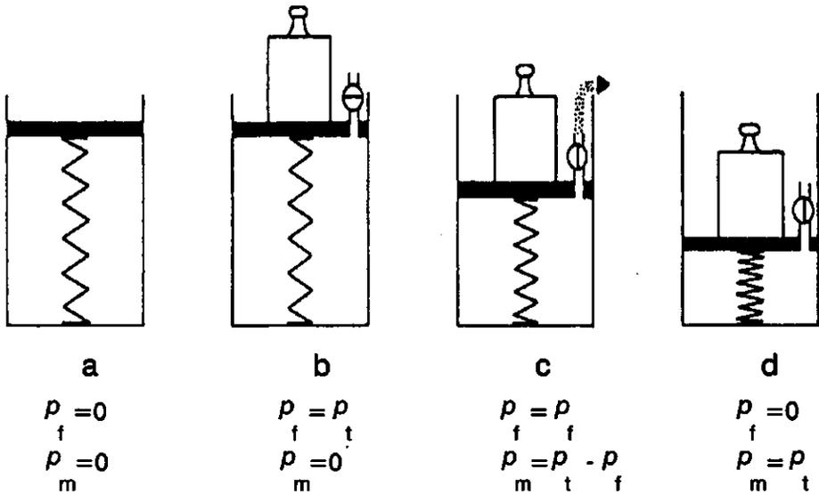
Fig. 1.5 The Terzaghi model, explained by a frictionless piston in a cylinder filled with an incompressible liquid, a spring, a stopcock and a load. In (a) a spring is immersed in a cylinder filled with water. In (b) a load is applied. The piston cannot descend and the liquid pressure is equal to the applied pressure. In (c) the stopcock is opened, water escapes and the piston sinks. At (d) the spring carries the total load (Van den Bijgaart 1988).
