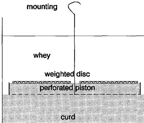
Fig. 2.6 A drawing of the apparatus to measure the stress needed to break the bonds between curd grains. The curd grains in the top layer fuse with the curd in the bottom layer at the openings in the perforated piston. The force needed to separate both layers is recalculated to a fracture stress. A filter paper, with holes congruent to those in the piston, was glued to the bottom of the piston to avoid adherence of curd to it. The glue becomes unstuck in the wet environment.
