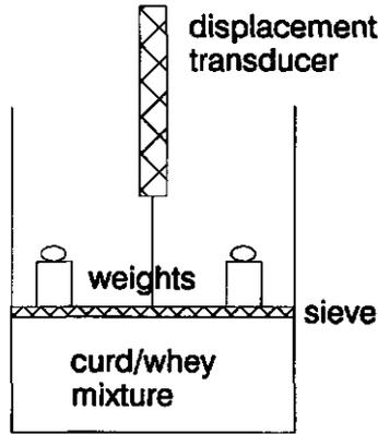
Fig. 1.6 Schematic representation of the compression tests as performed by Kerkhof (1979). A fairly thin layer of curd is compressed by means of a weight on top. The compaction is measured by means of a displacement transducer.
