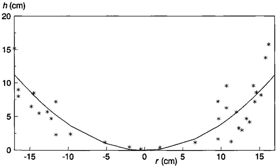
Fig. 4.6 The flow pattern of curd grains after drainage in a Casomatic drainage pipe.
