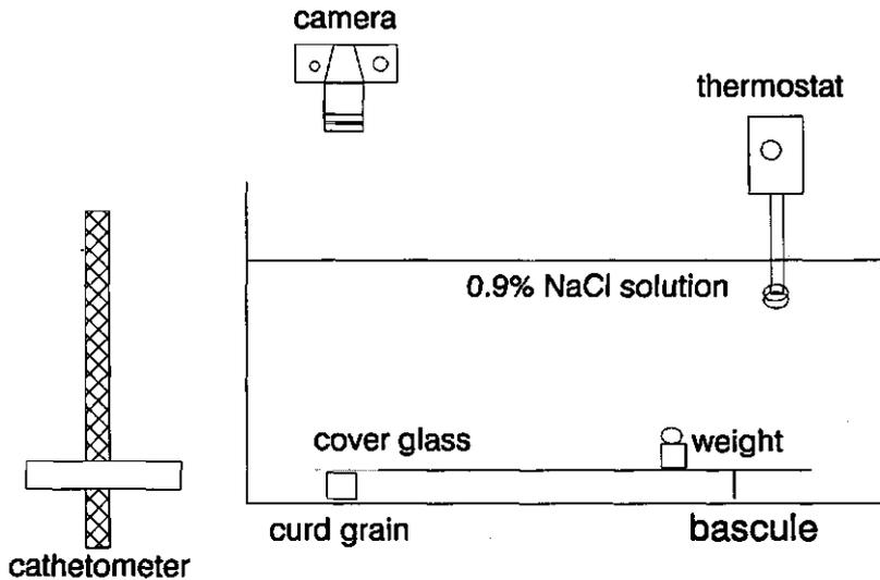
Fig. 2.2 A schematic drawing of the curd flattener.
