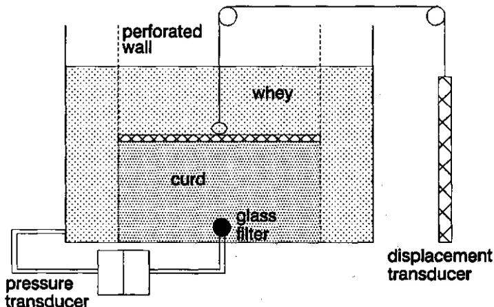
Fig. 2.3 A schematic drawing of the measurement of the liquid pressure and compaction of a curd-whey mixture in a cylindrical drainage column. The external pressure was exerted by applying a weight.
