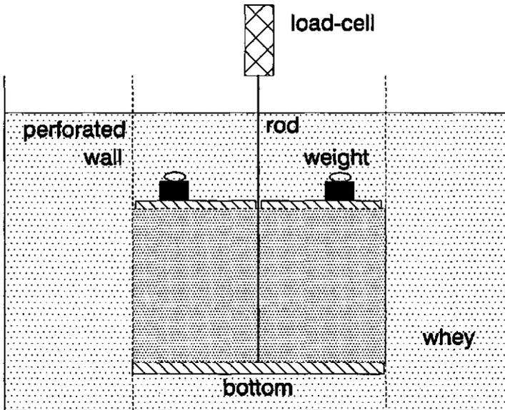
Fig. 2.5 A schematic drawing of the indirect measurement of the pressure loss in cylindrical drainage column. The load-cell has been mounted by means of a rod to the bottom of the curd bed. The exerted force on the bottom is less than the sum of the forces exerted due the weights and the curd layer. Its difference is due to adherence of curd to the wall.
