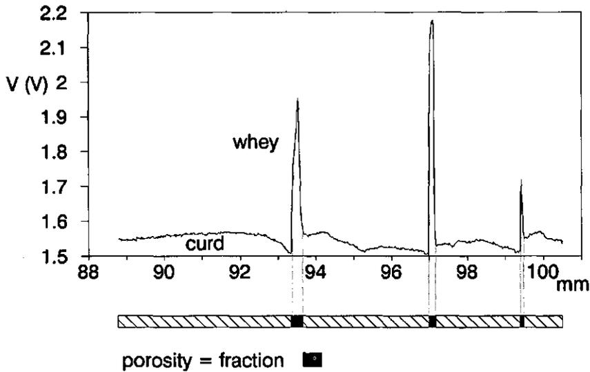
Fig. 2.8 Example of a part of the analogue signal of the photo-electric cell during a penetration in a curd bed. The conversion of the signal to a local porosity is also depicted.
