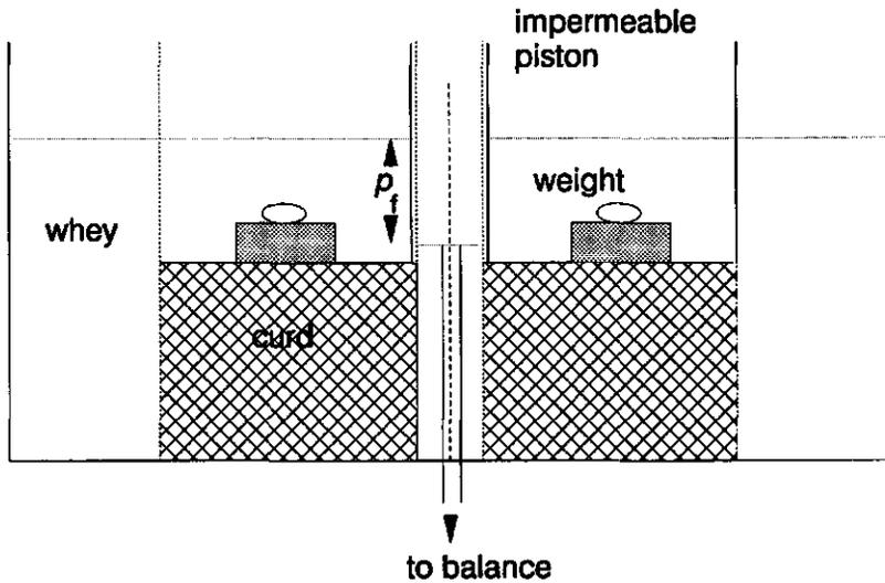
Fig. 2.4 The experimental setup of the radial permeability test.
