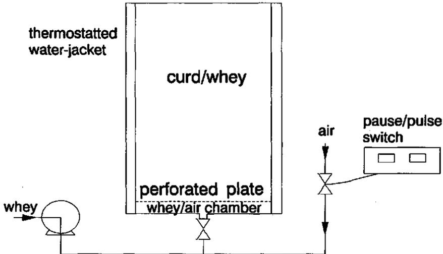
Fig. 2.1 A schematic drawing of the cheese vat used to prepare cube sized curd grains. The curd was clotted in the vat and cut into cube shaped particles; the latter were stirred by pumping whey and subsequently air through the bottom of the vat. The openings at the top of the whey/air distribution chamber were temporarily closed during clotting to avoid mixing of whey and milk.
