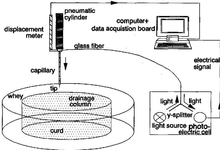
Fig. 2.7 A schematic drawing of the porosity meter.
