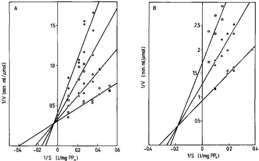
**Figure 4** (A) Inhibition of polyphosphate:AMP phosphotransferase by  $\text{P}_3$ . Symbols for  $\text{P}_3$  concentrations:  $\circ$ , 0 mM;  $\Delta$ , 0.97 mM;  $\square$ , 1.94 mM;  $*$ , 2.91 mM. (B) Inhibition of polyphosphate:AMP phosphotransferase by  $\text{P}_4$ . Symbols for  $\text{P}_4$  concentrations:  $\circ$ , 0 mM;  $\Delta$ , 0.61 mM;  $\square$ , 1.22 mM.
