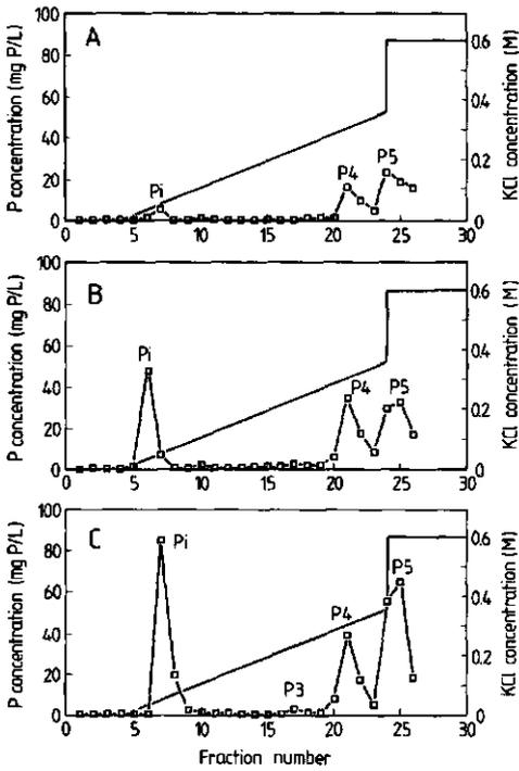
**Figure 2.** Degradation of high polymeric polyphosphate ( $n = 64$ ) by polyphosphatase followed by anion exchange column chromatography. A)  $t=0$ ; B)  $t=1$  hour; C)  $t=3$  hours. Orthophosphate ( $P_i$ ), triphosphate ( $P_3$ ), tetraphosphate ( $P_4$ ), and pentaphosphate ( $P_5$ ) are indicated.
