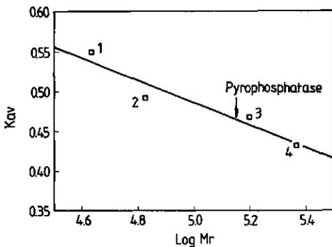
**Figure 1.** Molecular mass determination of the native pyrophosphatase on Superose 6 HR 10/30. Standards were ovalbumin (45 kDa, 1); bovine serum albumin (67 kDa, 2); aldolase (158 kDa, 3); catalase (232 kDa, 4). The position of pyrophosphatase of *A. johnsonii* 210A is indicated by the arrow.
