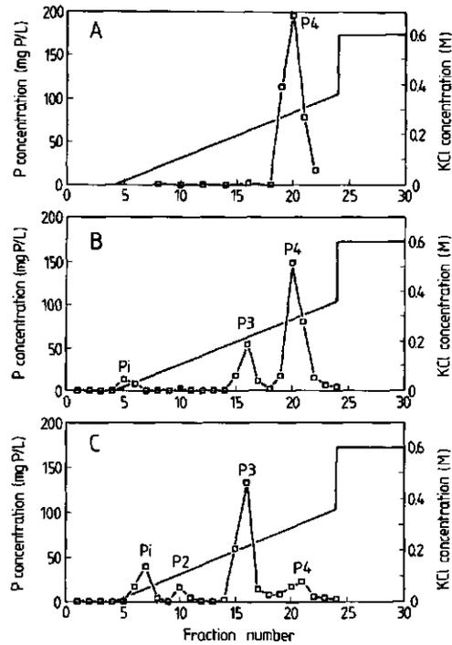
**Figure 3.** Degradation of tetraphosphate by polyphosphatase followed by anion exchange column chromatography. A)  $t=0$ ; B)  $t=2$  hours; C)  $t=3.5$  hours. Orthophosphate ( $P_i$ ), pyrophosphate ( $P_2$ ), triphosphate ( $P_3$ ), and tetraphosphate ( $P_4$ ) are indicated.
