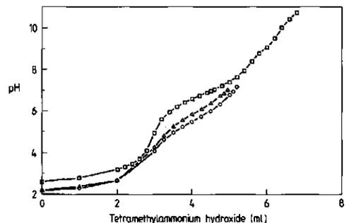
**Figure 3.** Titration of polyphosphoric acid with 0.1 N tetramethylammonium hydroxide.  $\square$ , polyphosphoric acid;  $\Delta$ , polyphosphoric acid +  $CaCl_2$ ;  $\circ$ , polyphosphoric acid +  $MgCl_2$
