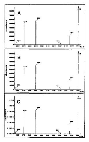
Fig. 4.4. Mass (MID) spectra of the purified major deconjugated metabolite of  $\beta$ -nortestosterone generated by pig hepatocytes (A), a standard of  $15\alpha$ -hydroxy-norandrostenedione (B), and a deconjugated metabolite with the same retention time in the urine of pigs, injected with  $\beta$ -nortestosterone (C).Compounds were derivatized with TMS, and the four major fragment-peaks were selected for comparison (MID).
