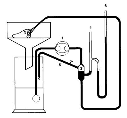
Fig. 2.1 Schematic presentation of the perfusion during the recirculation step with collagenase. The buffer is pumped by a peristaltic pump (1) via the oxygenator (2) to the liver sample (3), which is placed in a Büchner funnel. Oxygen is added via the oxygenator at (4) and escapes via the overload (5). The pressure is monitored with the manometer (6). All vessels containing buffer solutions, the oxygenator and the tubing are placed in a waterbath (40 °C).
