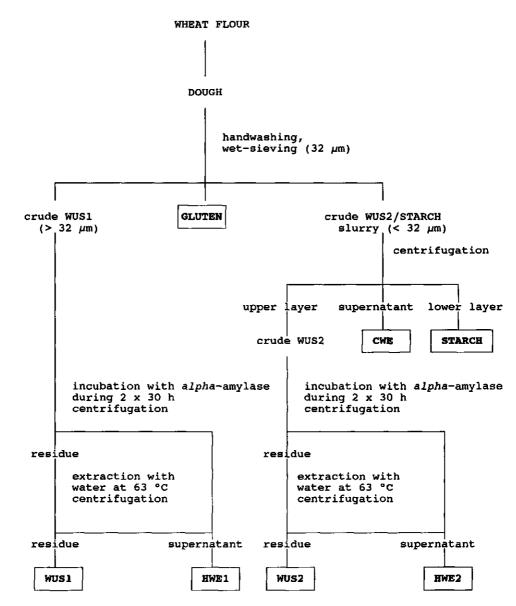
FIGURE 1. Fractionation procedure for the isolation of WUS from wheat flour.
