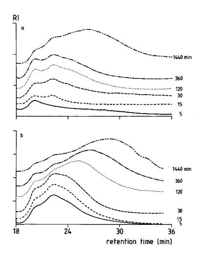
FIGURE 2. Elution pattern (HPSEC) of enzymic solubilized material from WUS by endol (a) and endoIII (b) after incubation times varying from 5 to 1440 min.
