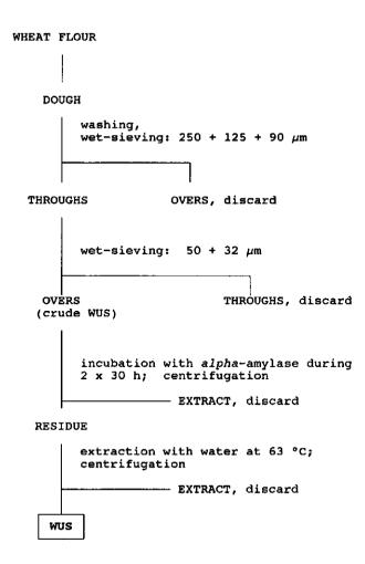
FIGURE 1. Schematic diagram for the large-scale isolation of WUS from wheat flour.
