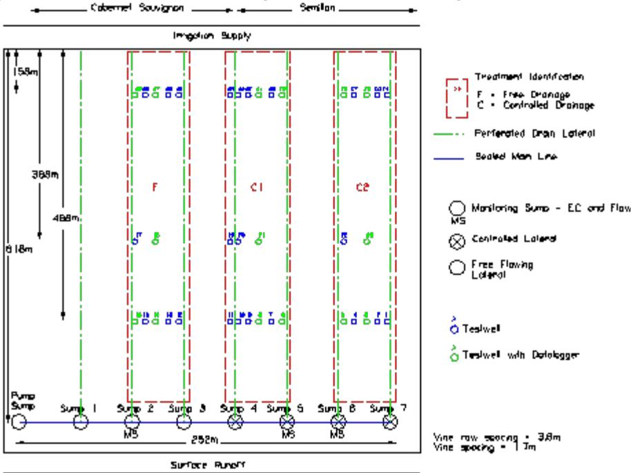
Figure 4 Experimental layout of field site showing drainage system and drainage treatments
