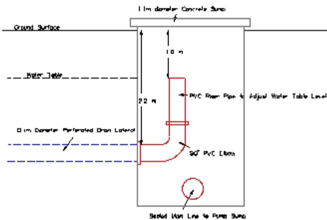
Figure 5 Cross-section of PVC pipe riser used as a weir for controlling flow and water tables
