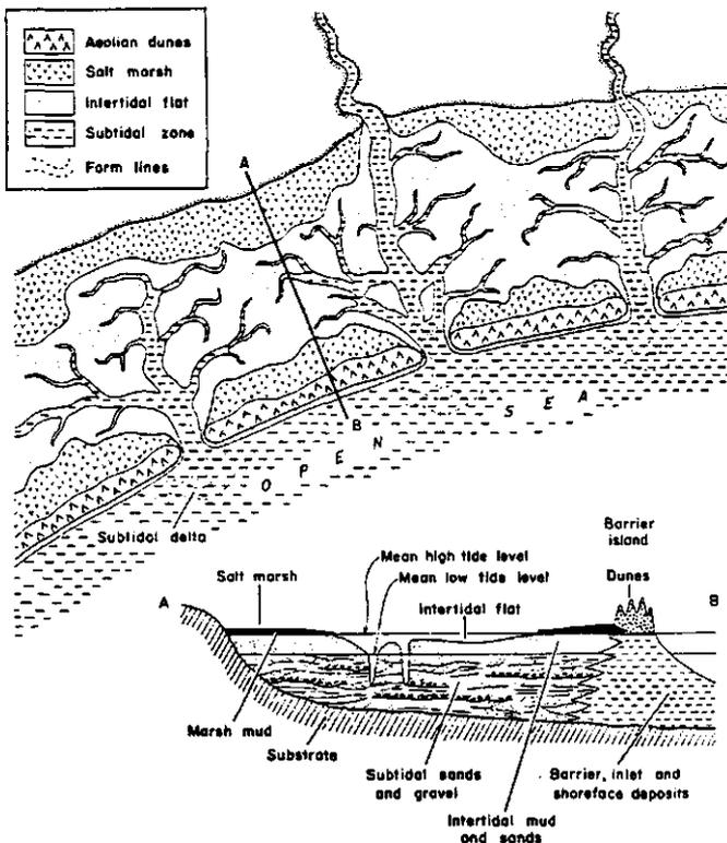
Fig. 4 Hydrology and morphology of a coastal lagoon (Allen 1970)
