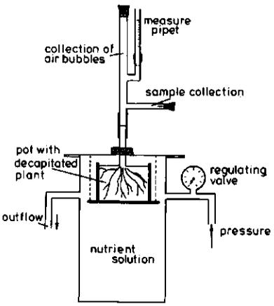
Fig. 4.6 Pressure bomb used to measure hydraulic conductance of roots.
