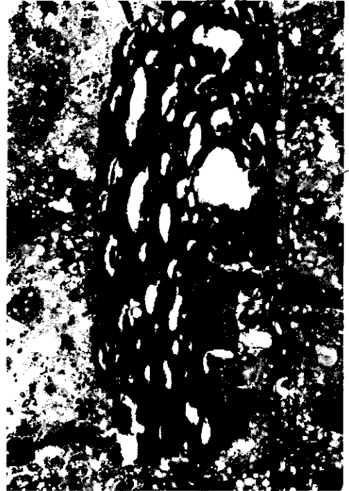
PHOTO 31. Charcoal in the mortar (photo width = 2.6 mm) (plain polarized light)
