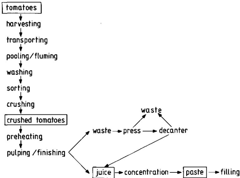
Fig. 2: Flow diagram for the production of tomato paste.
