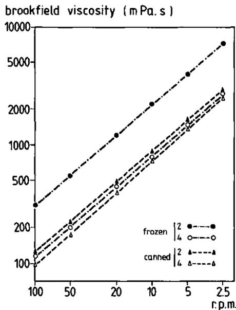
Fig. 9: Effect of pasteurization on gross viscosity of tomato juices reconstituted from paste. The hot break temperature was 100°C for sample 2 and 64.4°C for sample 4 (from Sherkat & Luh 1977).
