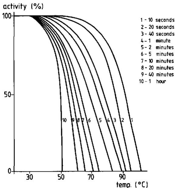
Fig. 6: Thermal inactivation of tomato PE
