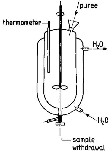
Fig. 38: Reaction vessel used for enzymatic treatment of diluted tomato paste.
