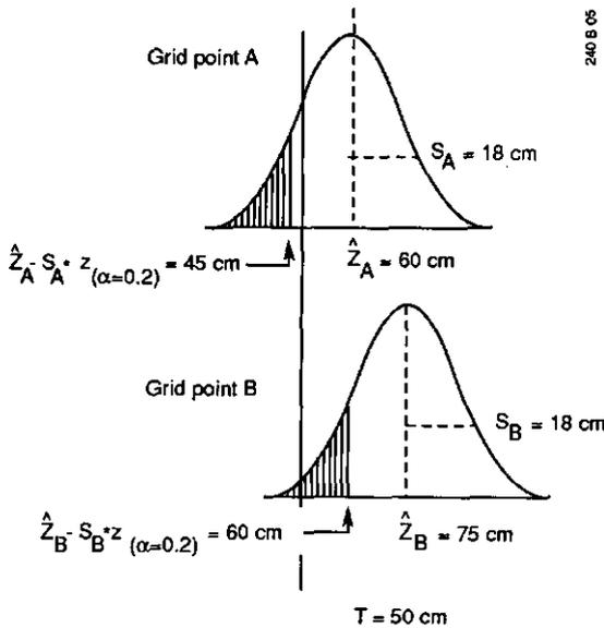
Fig. 8. Testing the condition of whether or not the true value of the variable at a grid point with a probability of 80% will exceed the threshold value of 50 cm.
