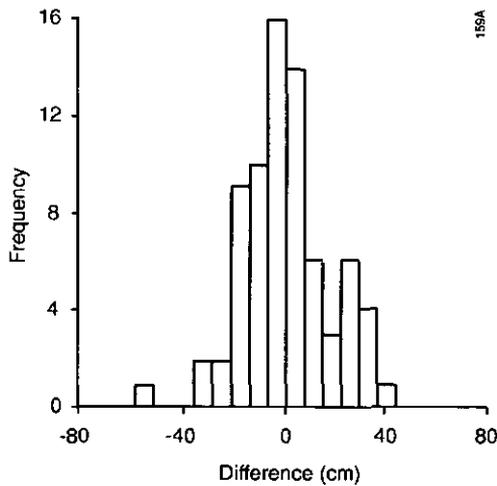
Fig. 7. Distribution of the prediction errors, calculated with inverse distance prediction to measured test points. The distribution has a mean of 0.06 cm and a standard deviation of 18.06 cm.
