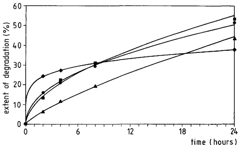
Figure 4: Influence of the pH and the buffer concentration on the rate of depolymerisation by  $\beta$ -elimination at 115°C: ■, 0.1M, pH 5.0; ●, 0.01M, pH 5.0; ◆, 0.1M, pH 6.0; ▲, 0.01M, pH 6.0.
