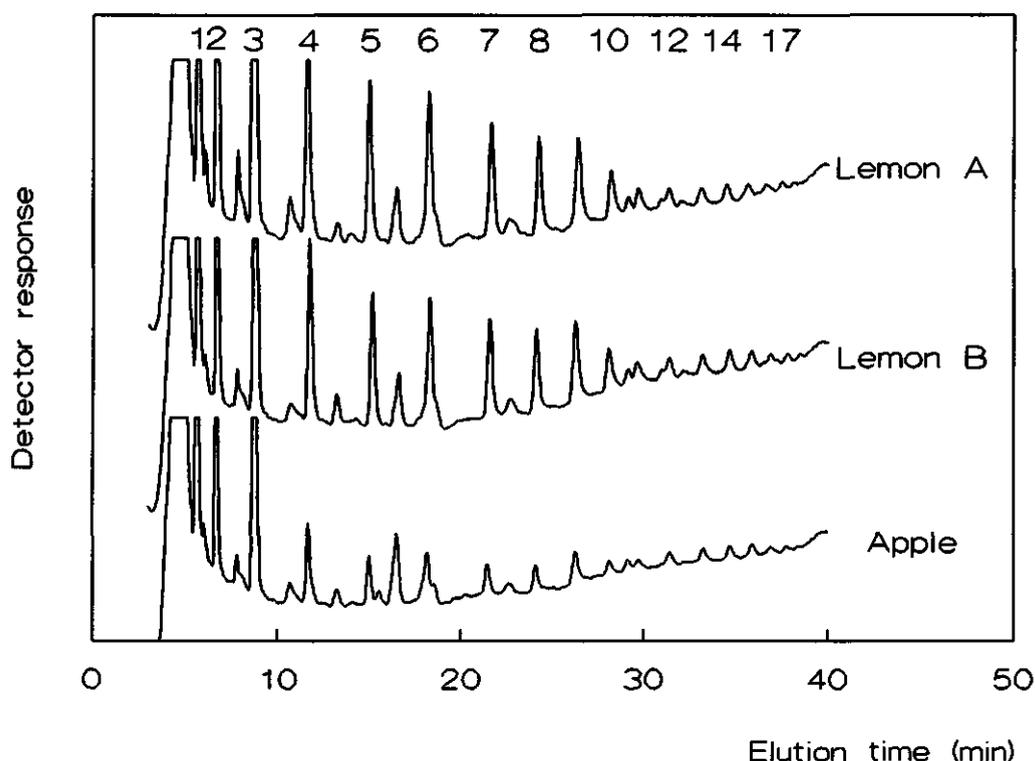
Figure 6: High performance ion exchange chromatography of the oligogalacturonides produced by the action of endoPG on the three pectin samples. Figures indicate the oligomer size.
