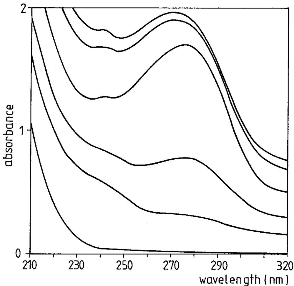
Figure 5: Changes in the UV spectrum of the reaction products of chemical  $\beta$ -elimination after 0, 4, 8, 24, 48 and 72 hours of treatment at pH 5 and 115°C.
