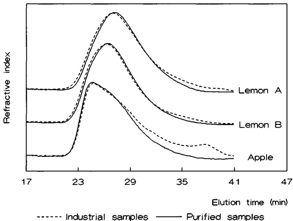
Figure 1: HPSEC of the industrial and corresponding Cu-purified samples
