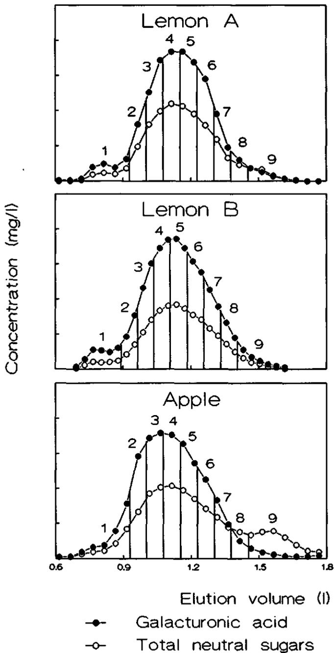
Figure 1: Elution patterns of the three industrial pectins on Fractogel TSK HW 55(S)/75(S) eluted with 0.1M Na-succinate buffer at pH 4.8 containing 29 mg/l of calcium cations.
