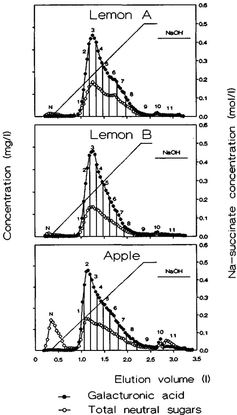
Figure 1: IEC elution pattern of the three industrial pectin samples on DEAE-Sephrose CL 6B.
