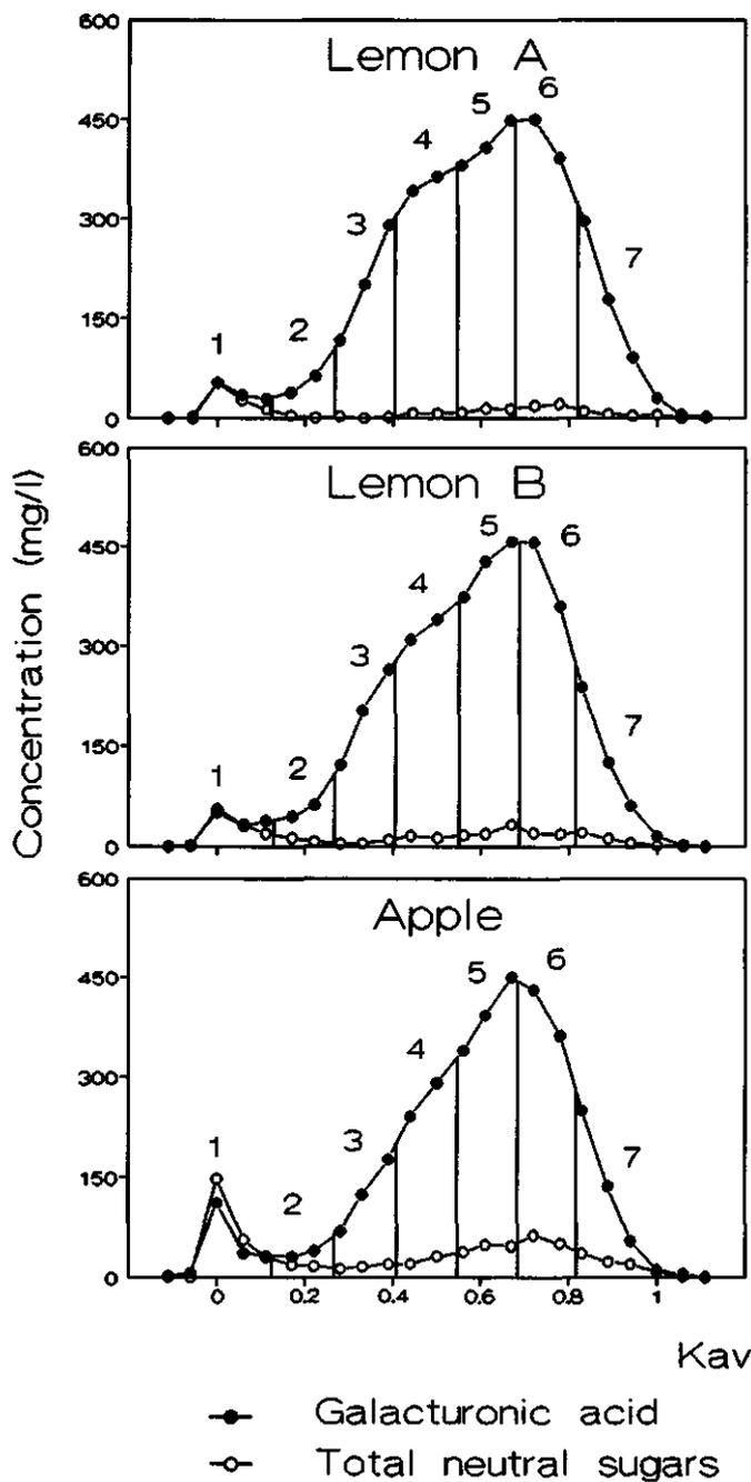
Figure 4: SEC elution pattern on Sephacryl S200 of the three purified pectin samples degraded by chemical  $\beta$ -elimination.
