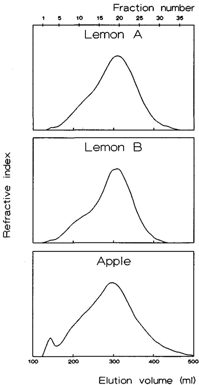
Figure 2: Elution patterns of the three industrial pectins on Sepharose CL-2B/Sepharose CL-4B eluted with 0.037M phosphate buffer at pH 6.5 with 0.001M  $\text{Na}_2\text{-EDTA}$ .
