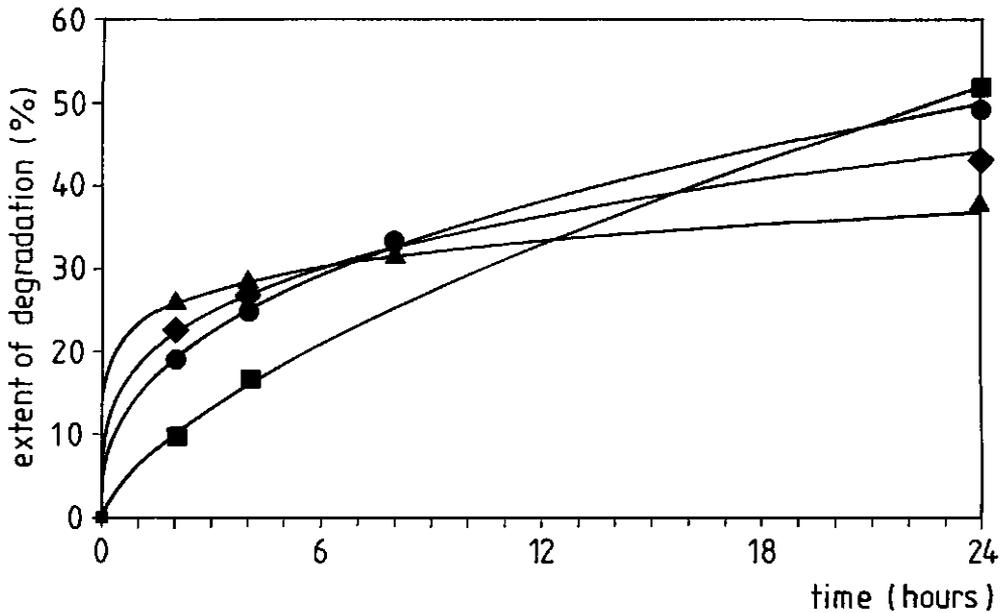
Figure 3: Influence of the pH on the rate of depolymerisation by  $\beta$ -elimination in 0.05M Na-citrate buffer at 115°C: ■, pH 5.0; ●, pH 5.4; ◆, pH 5.7; ▲, pH 6.0.
