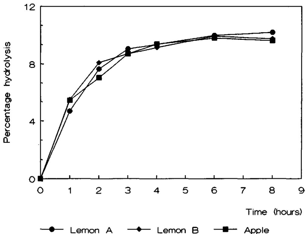
Figure 2: Rate of degradation of the three purified pectin samples by chemical  $\beta$ -elimination.
