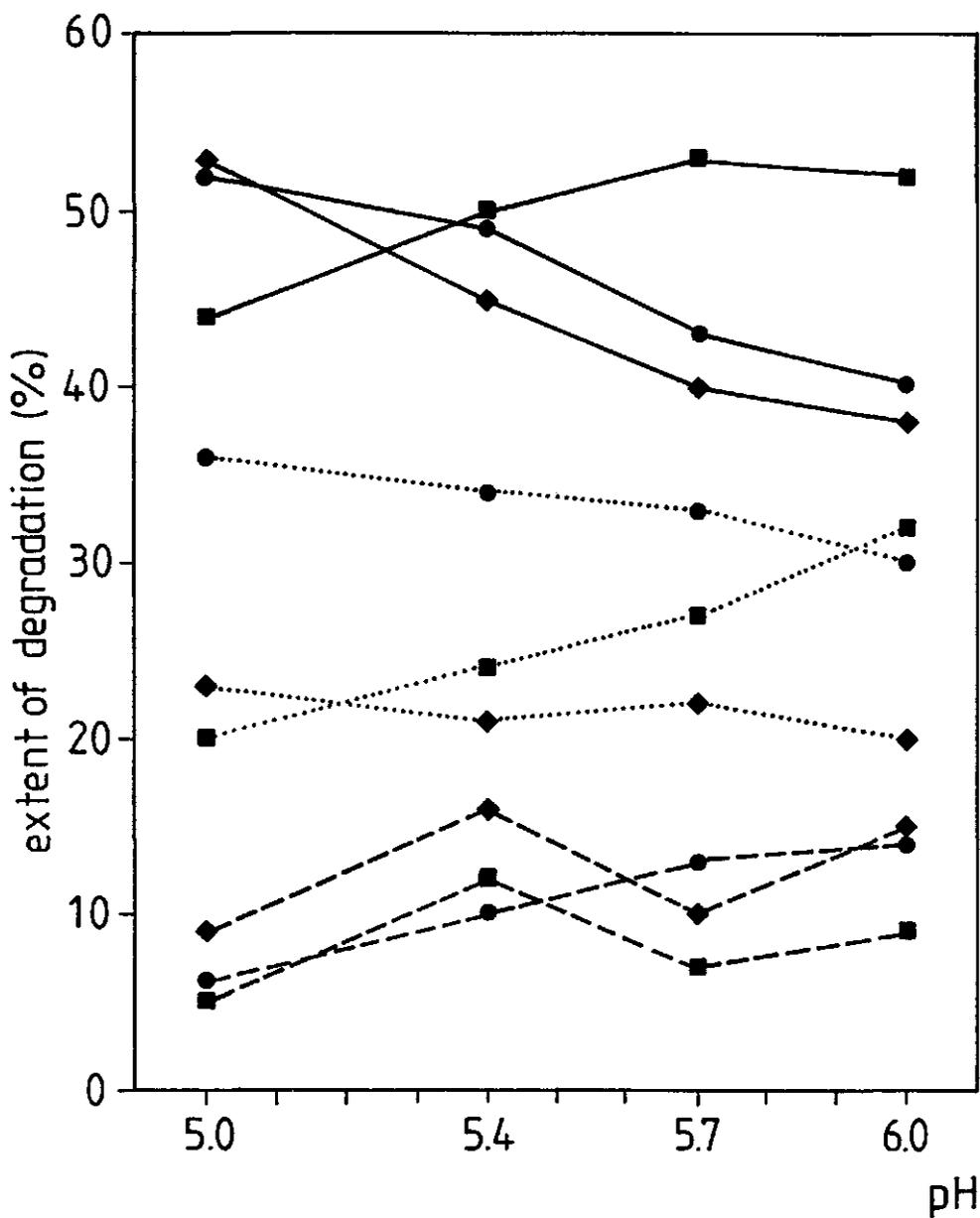
Figure 1: Extent of degradation after 24 hours of treatment in various conditions of pH, buffer concentration (■, 0.01M; ●, 0.05M; ◆, 0.1M) and temperature (---, 95°C; ····, 105°C; —, 115°C). Degradation is expressed as the percentage of split glycosiduronic linkages of all glycosiduronic acid linkages situated next to an esterified galacturonic acid unit.
