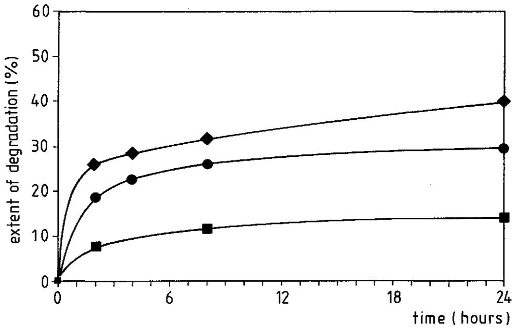
Figure 2: Influence of the temperature on the rate of depolymerisation by  $\beta$ -elimination in 0.05M Na-citrate buffer at pH 6.0: ■, 95°C; ●, 105°C; ◆, 115°C.
