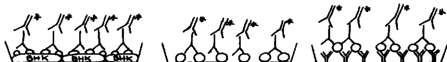
Fig 1. Illustration of three different radioimmunoassays to measure antibody. O=viral antigen, Y=anti-HSV-2-IgG, Y=antibody to be measured, Y* = I-labelled anti-mouse-Fab.
