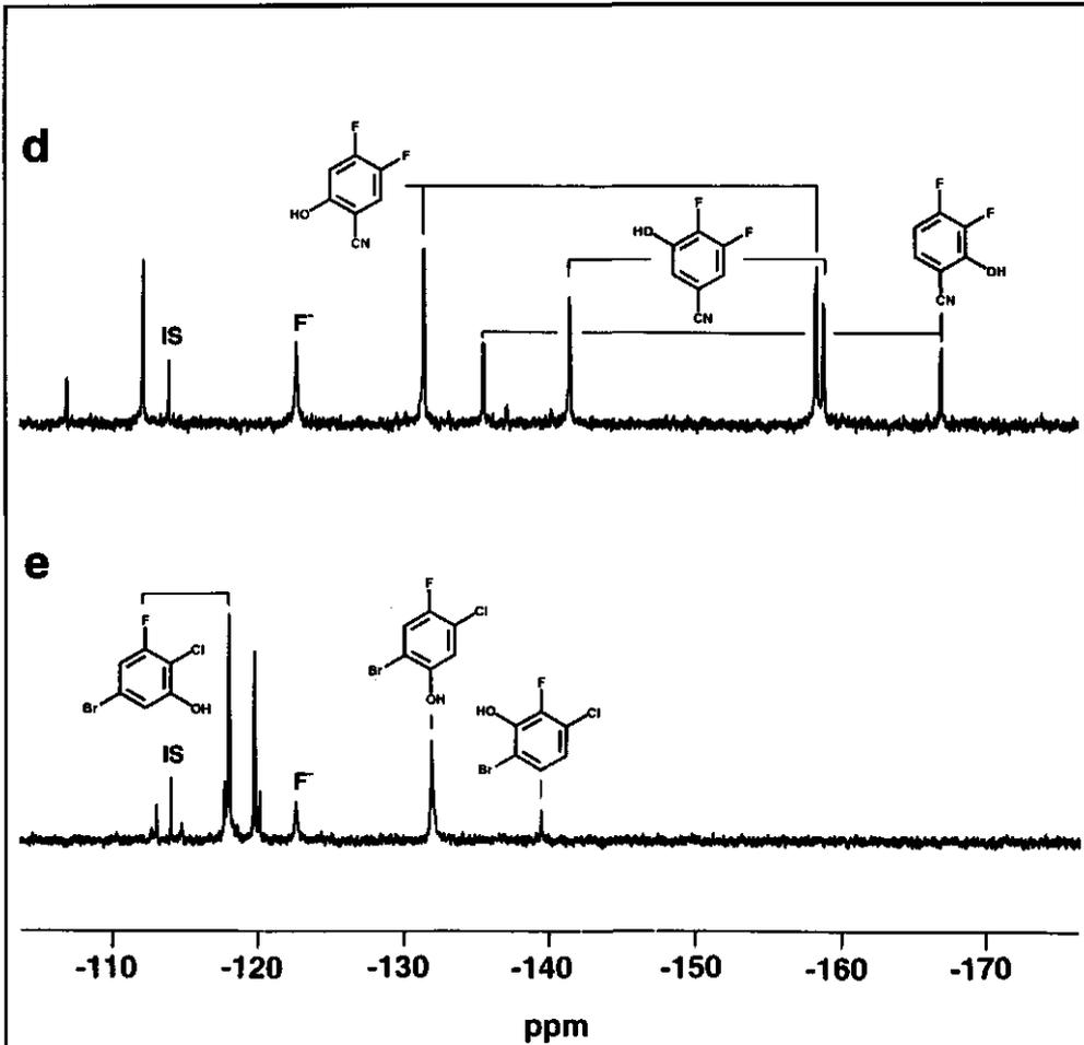
**Figure 2**  $^{19}\text{F}$  NMR spectra of the arylsulphatase/ $\beta$ -glucuronidase treated 0-24 h urine samples of rats exposed to (a) 4-chloro-1,2-difluorobenzene, (b) 4-bromo-1,2-difluorobenzene, (c) 4-iodo-1,2-difluorobenzene, (d) 4-cyano-1,2-difluorobenzene and (e) 2-chloro-5-bromofluorobenzene. The resonance marked "IS" is from the internal standard 4-fluorobenzoic acid.
