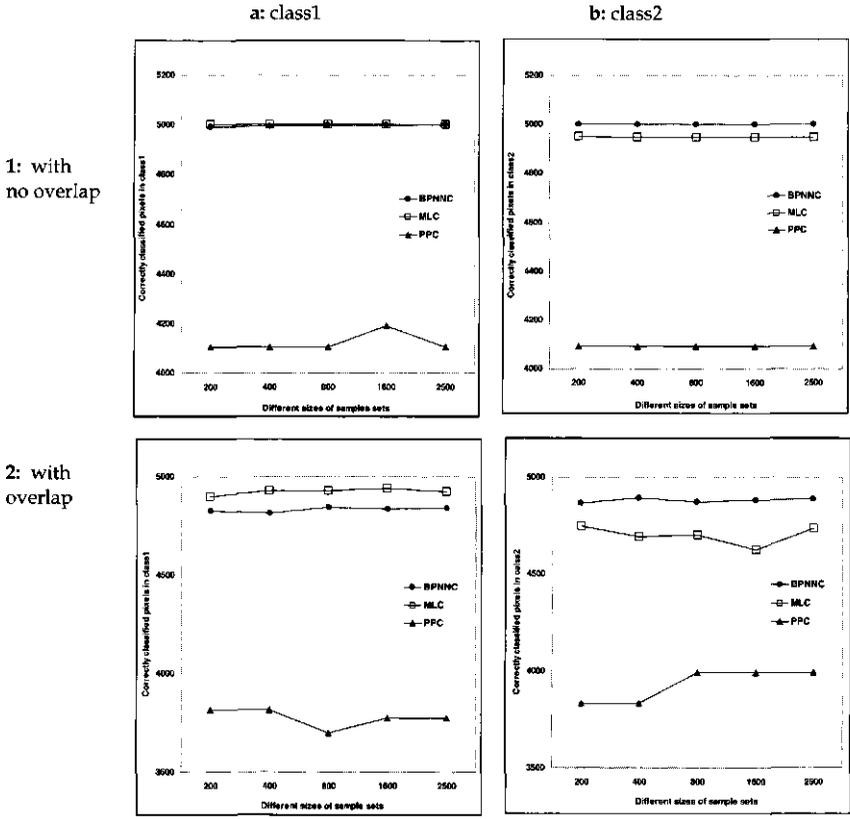
**Figure 2.6** Response of the backpropagation neural network classifier (BPNNC), maximum likelihood classifier (MLC) and parallelepiped classifier (PPC) to the different sizes of training sample sets for the simulated data sets. Note that BPNNC has a system error level of 0.005 for the “no overlap” situation and of 0.03 for the “overlap” situation.
