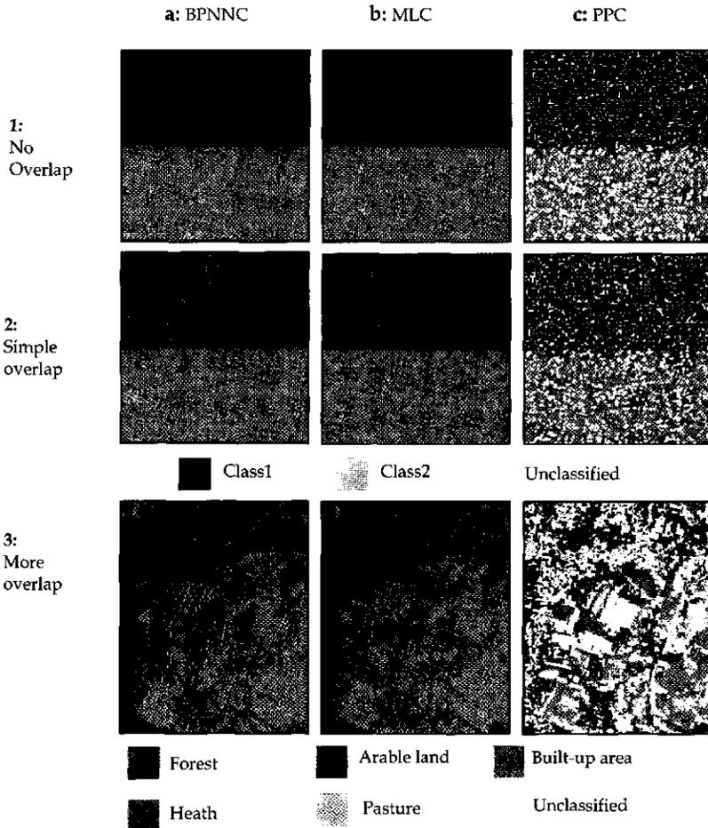
**Figure 2.7** The classified images from the backpropagation neural network classifier (BPNNC), maximum likelihood classifier (MLC) and parallelepiped classifier (PPC) for both simulated data sets and remotely sensed imagery. The left column is the outputs from BPNNC, the middle column from MLC, and the right column from PPC.
