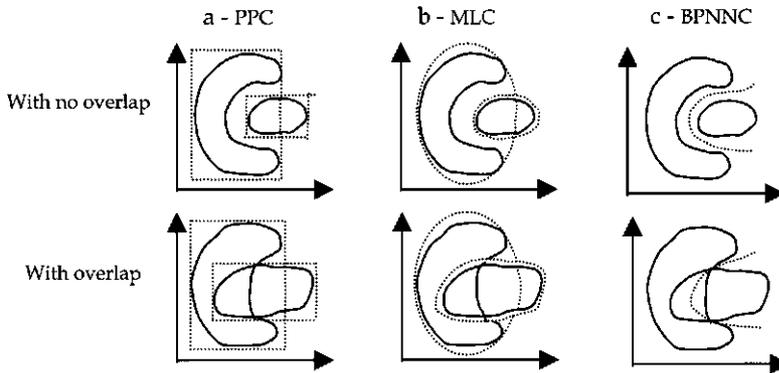
**Figure 2.1** Decision rules for the three different classifiers in a two-dimensional feature space (after Skidmore et al. (1988) and Richards (1995)). PPC, MLC and BPNNC represent the parallelepiped classifier, the maximum likelihood classifier and the backpropagation neural network classifier respectively.
