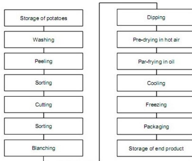
Figure 2: Scheme of French fries production process (Van Loon, 2005)
