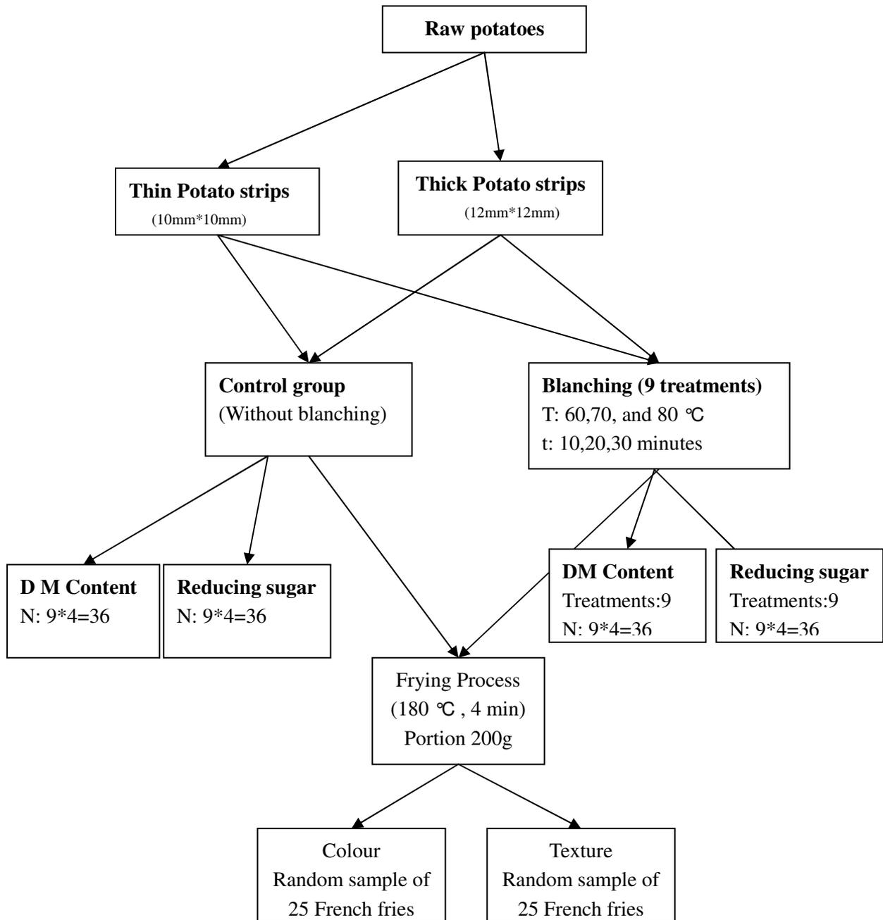
Figure 7: Schematic diagram of experimental process
