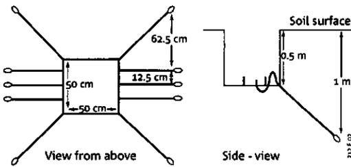
Fig. 4.2 Installation of suction cups for soil water sampling
