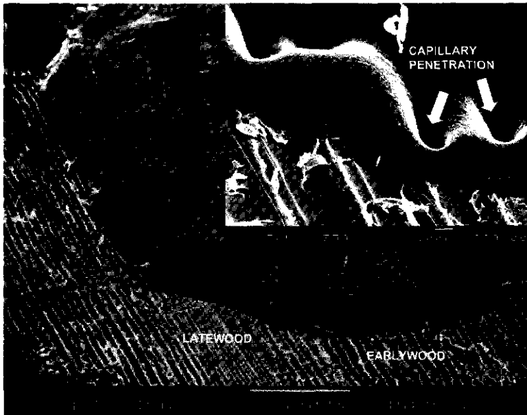
Figure 6.2 Microscopic image (SEM) showing influence of wood structure on the spreading of the coating droplet. Insert at higher magnification shows substrate penetration in the spreading liquid front.
