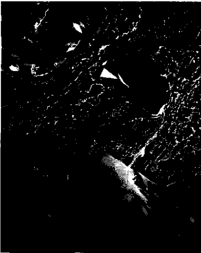
Figure 2.9 SEM-microphotograph (200 x) showing how the SBA coating is resting on the membrane of a tylose (arrow) in a half open cut vessel in meranti.
