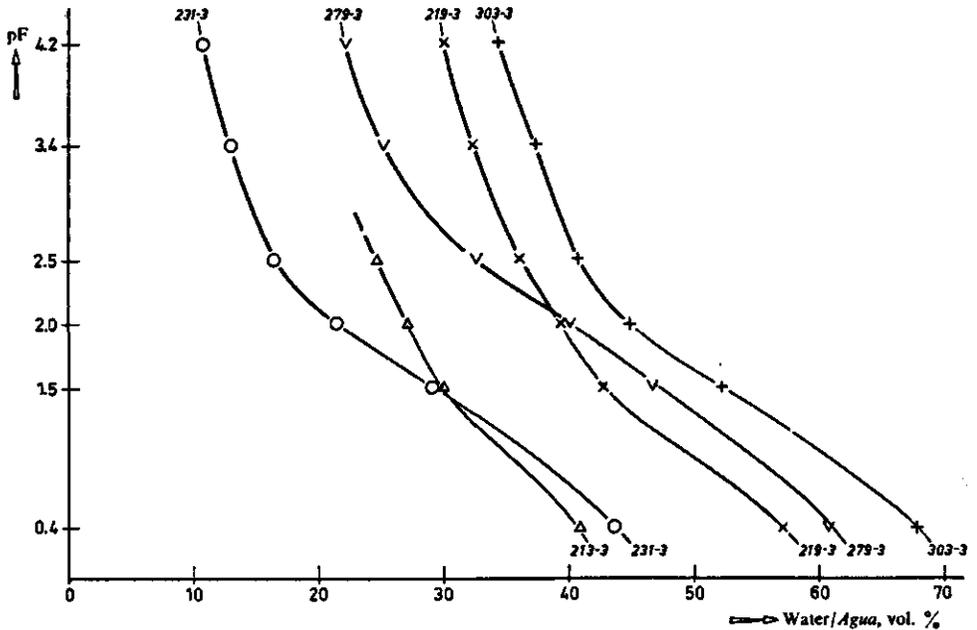
Fig. 37 Moisture tension curves from samples of a number of freely kaolinitic Planicie soils, and of some other Amazon soils. By courtesy of the Institute for Land and Water Management Research (I.C.W.) of Wageningen, Holland
