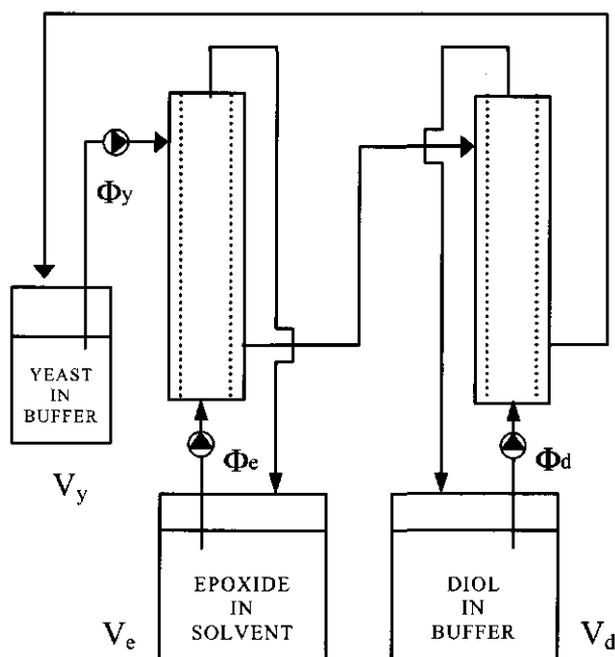
**Scheme 2.** Schematic diagram of a two-phase cascade membrane bioreactor for batch-wise epoxide resolution.
