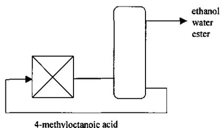
**Figure 2:** Scheme of the esterification of 4-methyloctanoic acid with ethanol in a packed bed reactor filled with Novozym 435<sup>®</sup>. The reaction mixture is fed into a strip column or distillation column to remove the ester from substrate phase.
