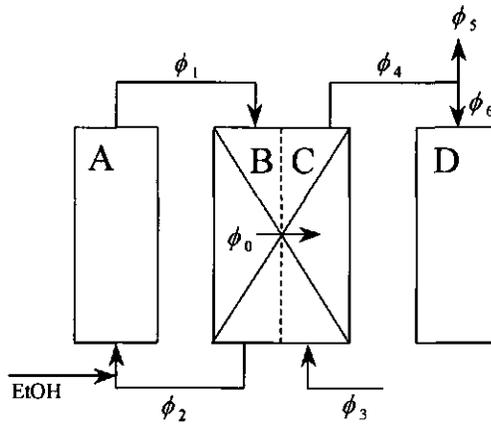
**Figure 5:** Simulation model for the integrated esterification of 4-methyloctanoic acid in a trickle bed reactor and separation of the produced ester from the reaction mixture.
