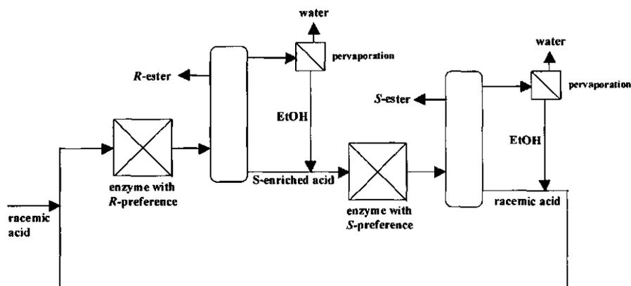
**Figure 3:** Proposed system for the production of 4-methyloctanoic acid ethyl ester with a high enantiomeric excess of the product. Two enzymes with the opposite enantiopreference are integrated into the system.
