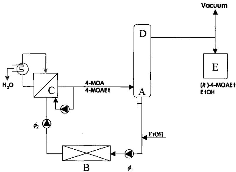
**Figure 8:** Esterification of 4-methyloctanoic acid with ethanol at 35°C in a packed bed reactor (B), containing Novozym 435<sup>®</sup> and distillation of the ethyl ester from the liquid phase (A) to the vapor phase (D).  $V_B$ :  $3.4 \cdot 10^{-5} \text{ m}^3$ ;  $\phi_1$ :  $7.4 \cdot 10^{-10} \text{ m}^3 \text{ s}^{-1}$ ;  $\phi_2$ :  $5.5 \cdot 10^{-8} \text{ m}^3 \text{ s}^{-1}$ .
