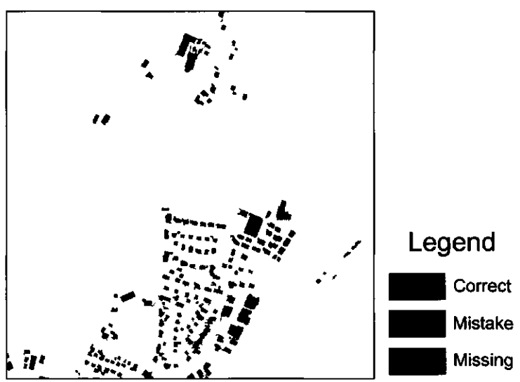
Figure 6.16: Comparison of extracted buildings as shown in Figure 6.13 with the reference data of Figure 6.14, Ravensburg, Germany.
