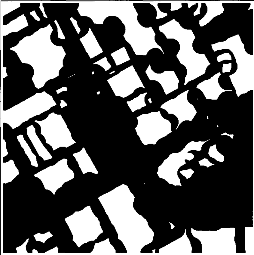
Figure 7.28: The solid interiors of clusters created by the morphological closing operation using 100 m as radius for the circular SE.
