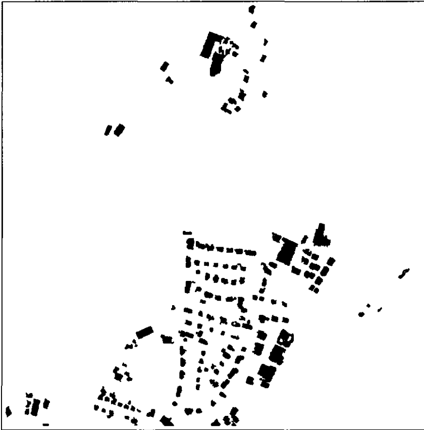
Figure 6.12: Building extracted by using 30 % as threshold for checking the size differences and using fuzzy membership functions based on other features, Ravensburg, Germany.
