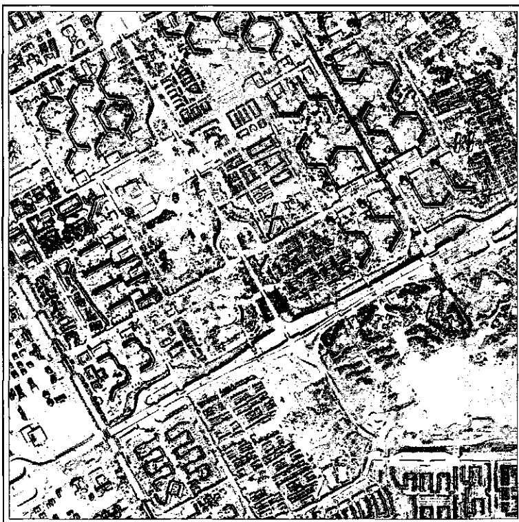
Figure 6.25: Simulated shadow areas of buildings by hillshade analysis based on laser data.
