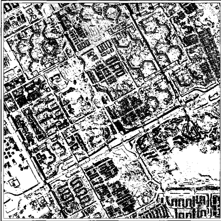
Figure 6.26: Simulated building relief displacement by hillshade analysis based on laser data.
