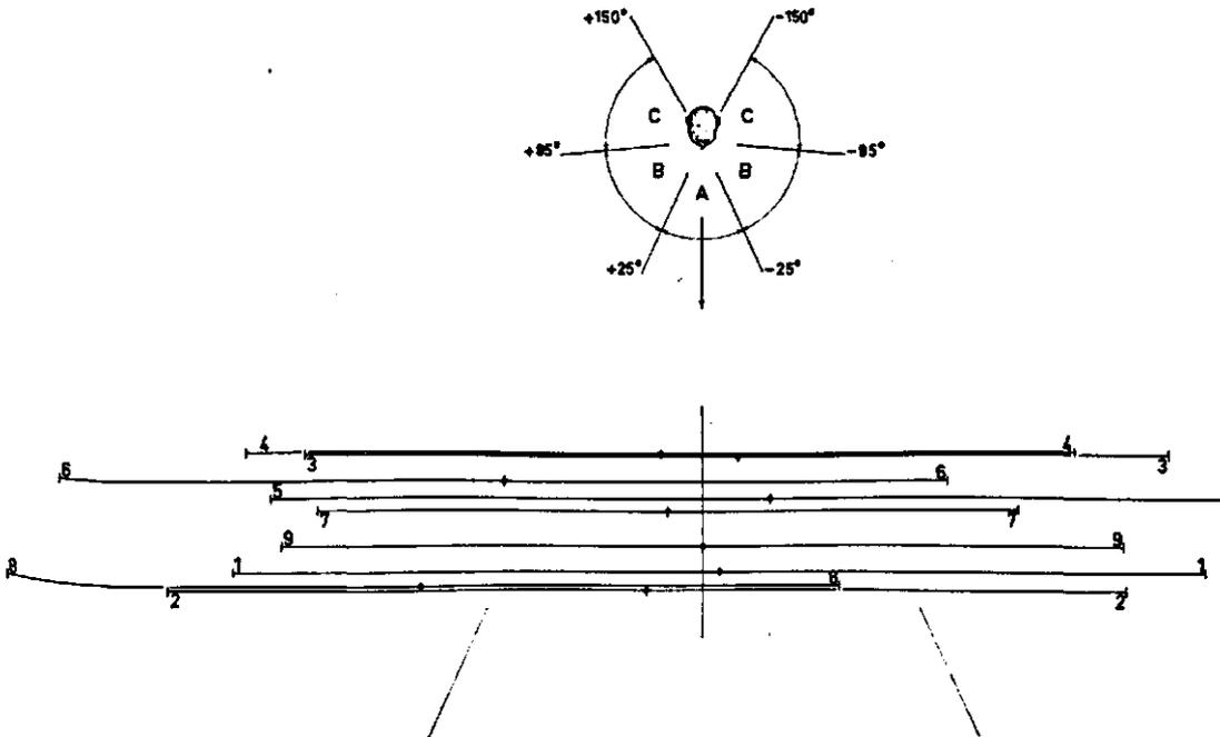
FIG. 13. Visibility of the cutterbar on combines (horizontal plane).
