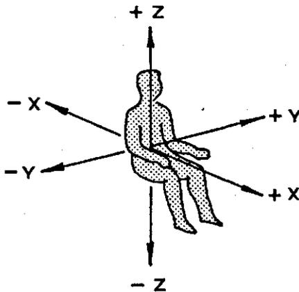
FIG. 17. System of coordinates for mechanical vibrations (I.S.O.; 1967).
