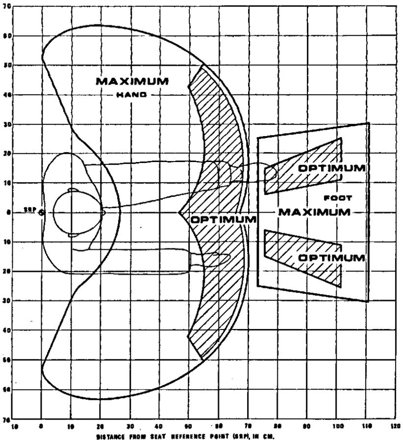
FIG. 4<sup>a</sup>. Optimum work-space lay-out for a self-propelled combine harvester (horizontal plane); 18 cm above seat-reference point (SRP).
