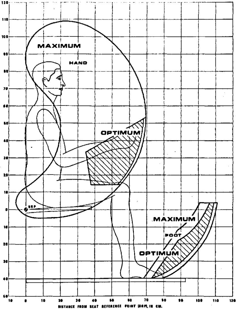
FIG. 4<sup>b</sup>. Optimum work-space lay-out for a self-propelled combine harvester (vertical plane). SRP – seat-reference point
