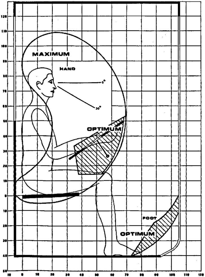
A.2. Optimum work-space lay-out for the self-propelled combine harvester (vertical plane).
