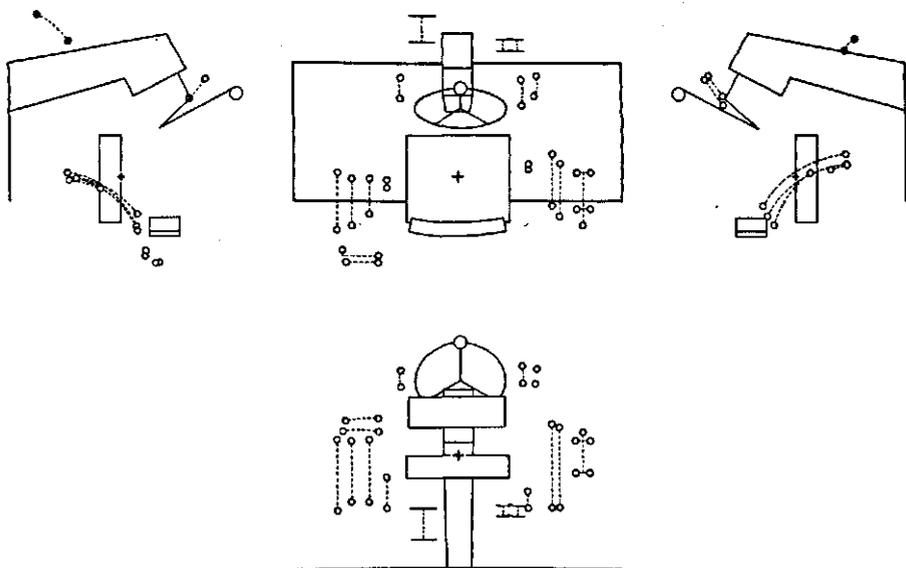
FIG. 6. Work-space lay-out of a self-propelled combine harvester.
