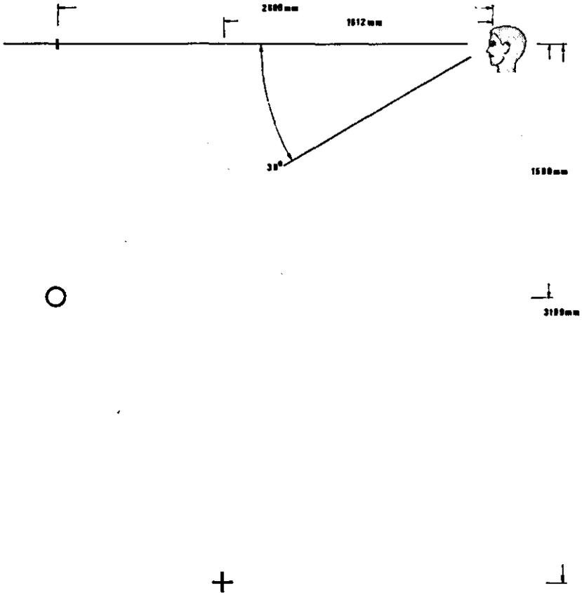
FIG. 28. Optimum visibility of the cutterbar for the self-propelled combine harvester (vertical plane).
