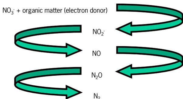
Figure 1: The denitrification process.
