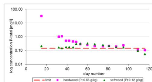
Figure 3: Phosphorus in leachate from hardwood and softwood chips. Especially in the beginning concentrations are high
