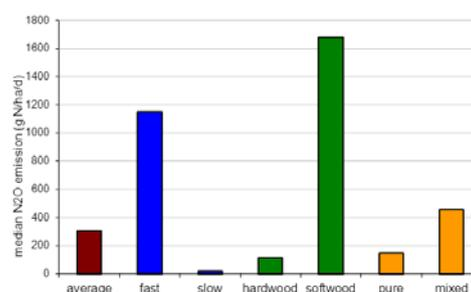
Figure 2: Influence of percolation speed, type of woodchip, and mixing with sand on emission of  $\text{N}_2\text{O}$  from woodchips
