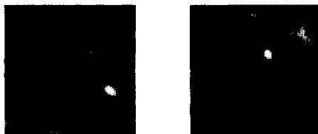
Figure 3.4: Correlation coefficient as a function of azimuth and range translation for X-band (left) and C-band (right). A clear global maximum can be identified in both correlation images (white dot). The size of both images is 130 lines (horizontal) by 130 pixels (vertical).
