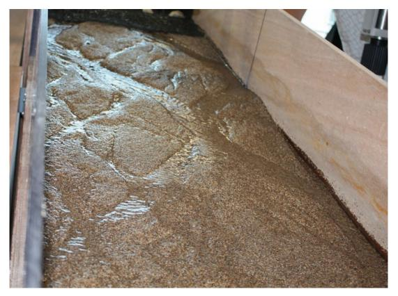
Figure 3.2 Rill development during an experimental run.
