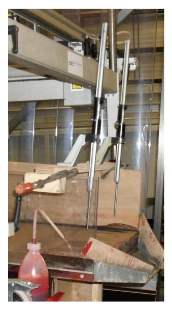
Figure 7.1 Side view of the installed point gauges for flow depth measurements
