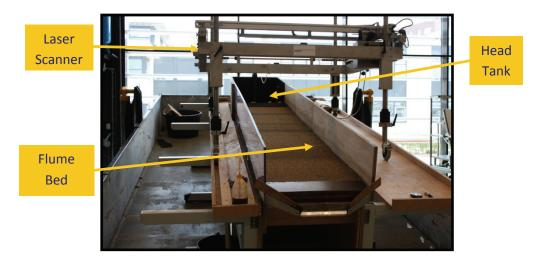
*Figure 1.1 Experimental flume utilized for the measurements of hydraulic and sediment parameter.*
