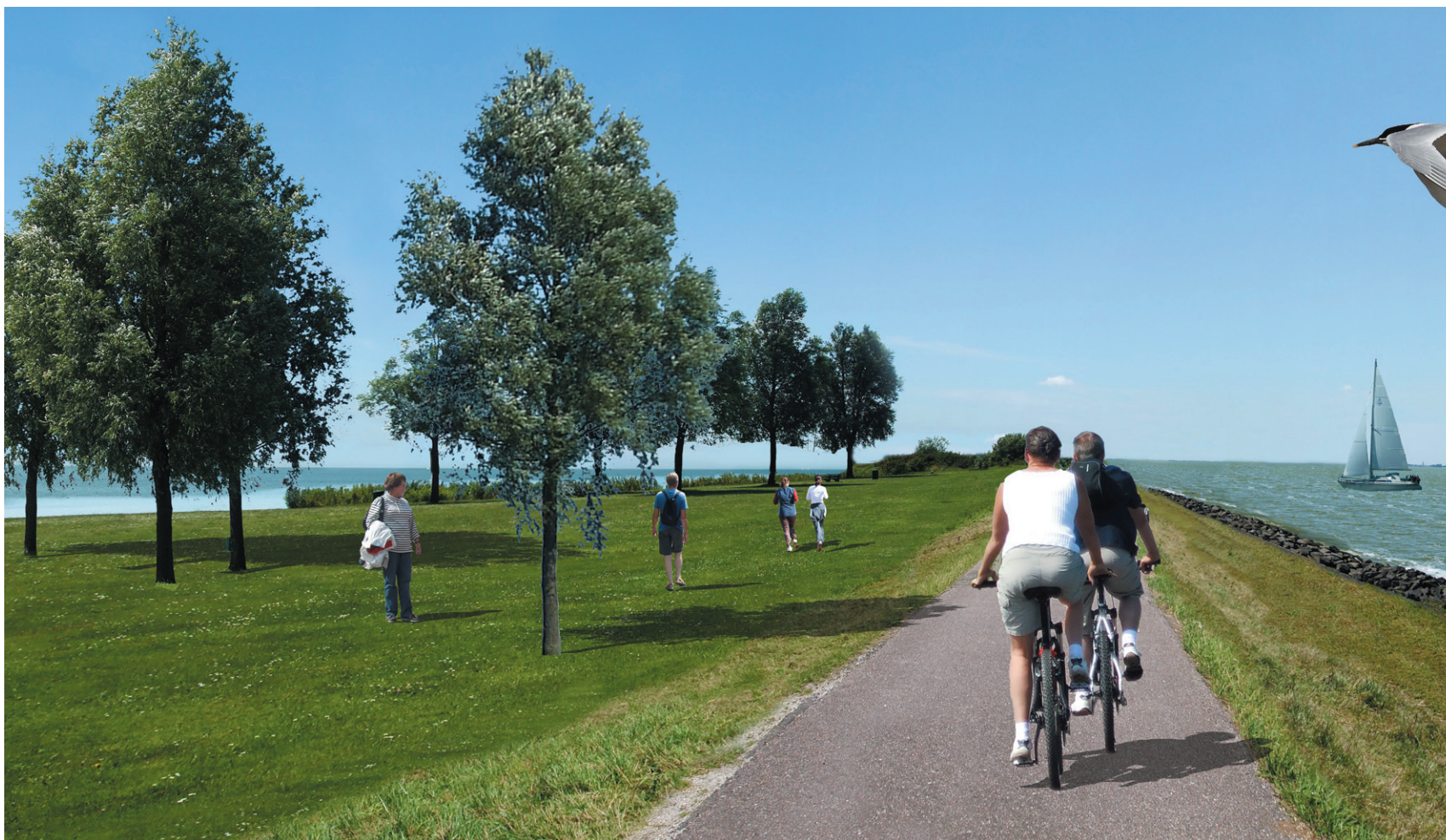
Figure 7.17a: visualisation of the dam in front of Enkhuizen. The dam will be accessible for cyclists and walkers, and also for cars with a maintenance function. The area on the side of the new lake will be mainly a grass area with some trees spread around, so that it will look quite open. Also a small beach will be created. On the IJsselmeer side the dam will run straight into the lake, so that boats can come close to the dam.
