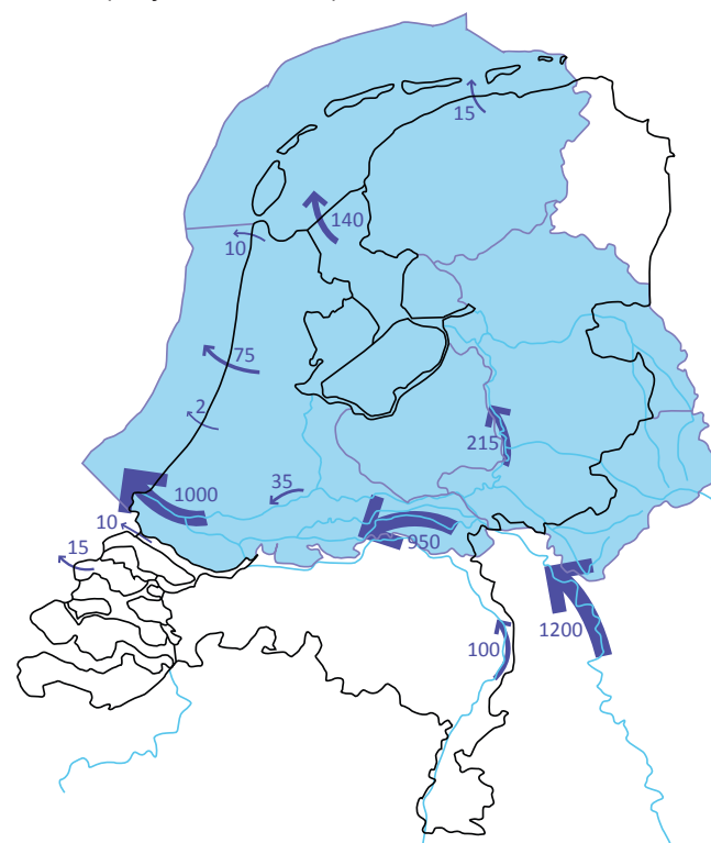
Figure 2.7: Rijndelta sub area with fresh water supply and drainage in the Netherlands in m³/s during the normal supply of 1200 m³/s through the river Rhine (based on: Rijksoverheid, 2008 and Projectteam, 2009)
