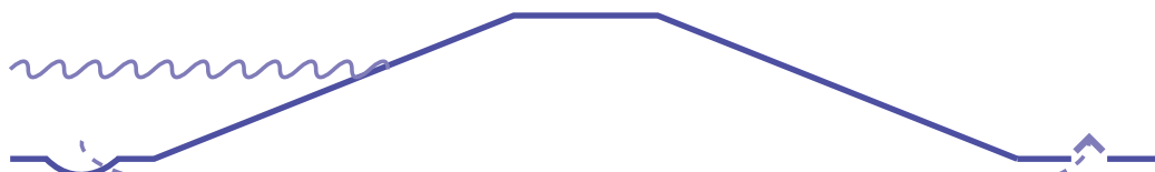
Figure 5.2d: fail mechanism: piping due to internal erosion (5.2a-d based on: Feddes et. al., 1988)
