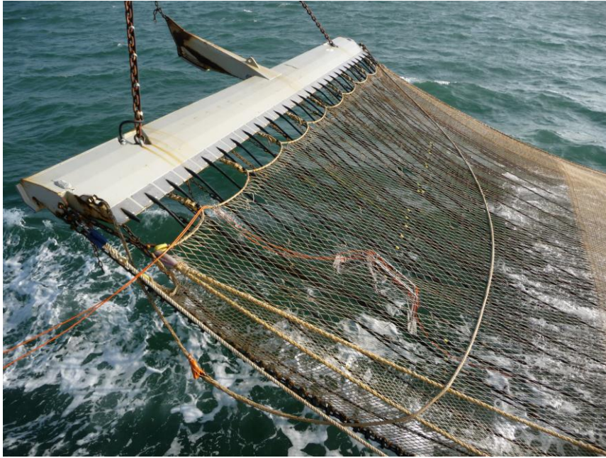
Figure 19 The rigid frame carrying three field strength probes and an DeepSea 1060 underwater video camera clamped on the first conductor pair of field 5 and 6 of the HFK PulseWing system on-board OD17 (1470 kW licenced vessel).
