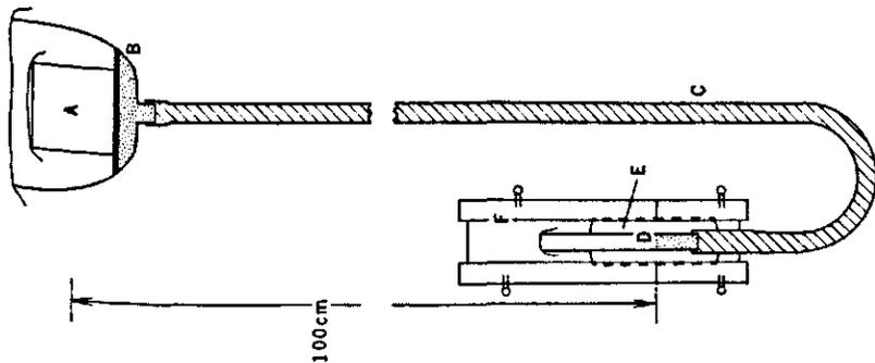
Fig. 40. Apparatus for estimating soil permeability. A = soil sample in steel cylinder of 100 cc; B = porous plate; C = rubber tube filled with water; D = glass tube with scale; E = segment with D, movable along F.
