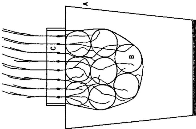
Fig. 51. Experiments of series 1. A = plastic container with some water on the bottom; B = soil balls; C = plastic ring with moist sand and young wheat plants.
