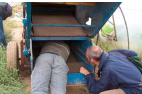
It is important to clean out machines thoroughly before moving on to the next variety
