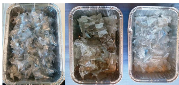
Figure 7: Photos of the PET bottle material. The cleaned PET material is shown on the left and a comparative photo between the non-treated and treated PET is shown on the right.
