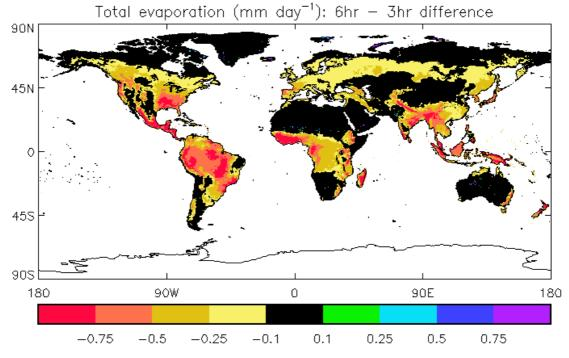
Figure 8: Differences in global mean total evaporation from (a) three hour – one hour model timsetep, and (b) six hour – three hour model timestep
