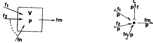
Fig. 7 Physical model (left) and bond graph (right) of vapour storage with in- and outgoing flows.
