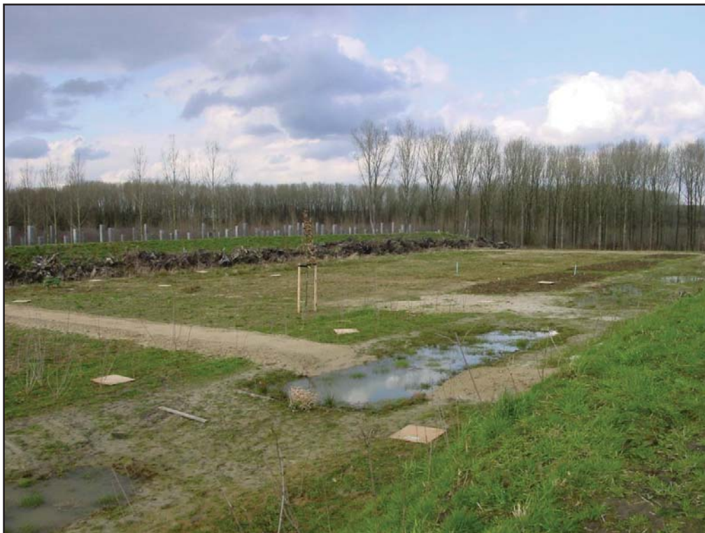
Figure 4. Wooden plates that were systematically spread out along the four transects functioned as artificial shelters which eased and standardised the counting of amphibians on the overpass. In the front the wetland zone with one transect on each side. In the back the dry zone with two transects as well, bordering the wall of tree stumps (Photo courtesy of E. van der Grift).
