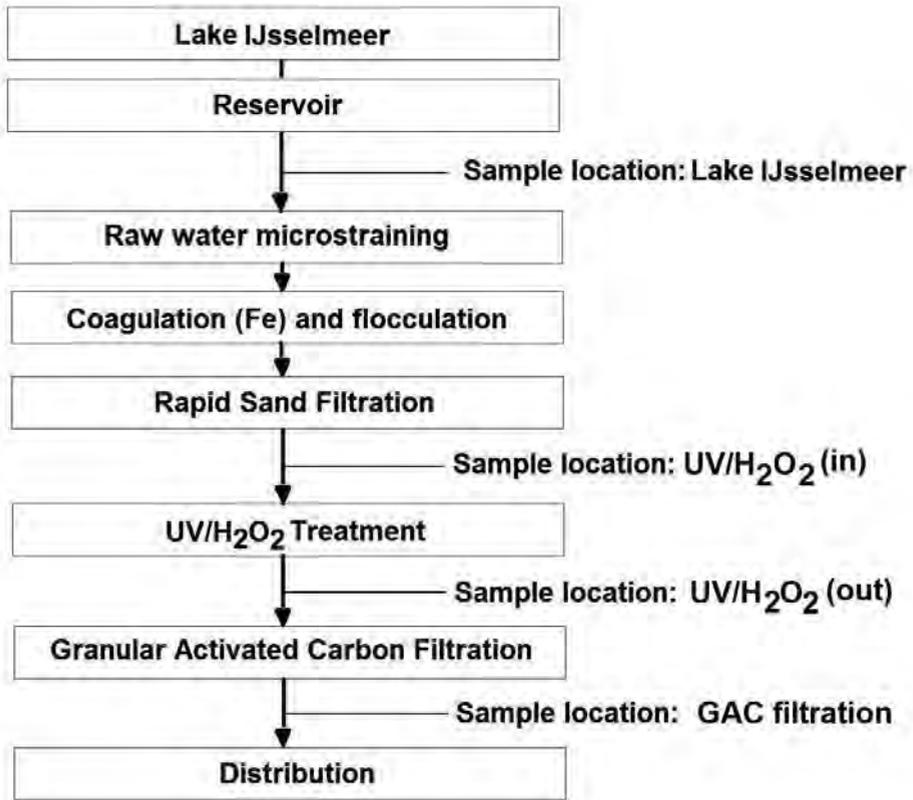
Figure 6.2: Water treatment process scheme of water treatment plant Andijk and sample locations.
