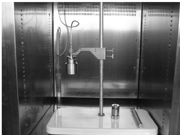
Figure 3. The probe and the sample holder in temperature controller
