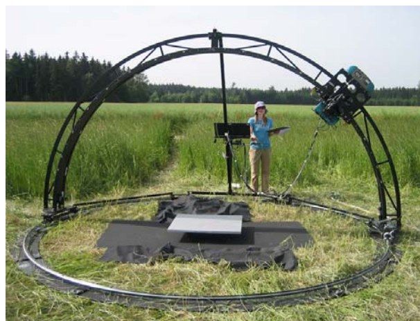
Figure 1. Dual field-of-view goniometer system FIGOS
