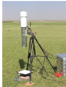
Figure 1. TerFlex sensor in its measuring configuration.
