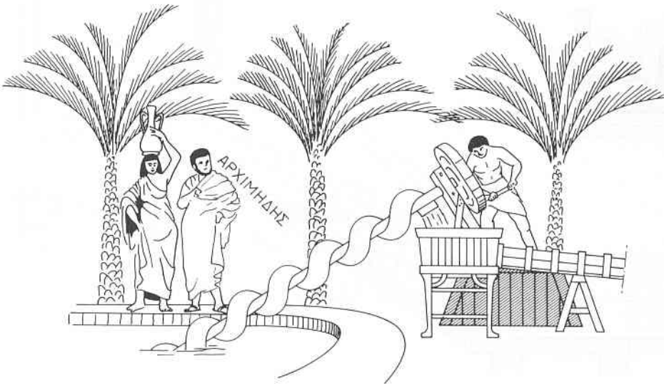
Figure 23.1 The ancient Archimedean screw
