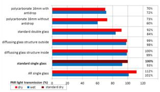
Transmission for PAR light of the tested cover materials, dry and wet; 100% is the standard single cover dry = 100% PAR light transmission
