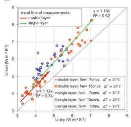
Ratio of the heat transfer coefficient (U factor) of the wet cover vs the corresponding value when dry
