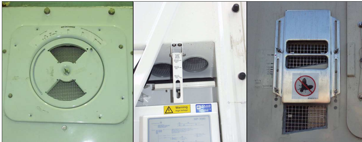
Fig. 3, some of the most common fresh air vents (from left to right Carrier, Thermo King, Daikin).
