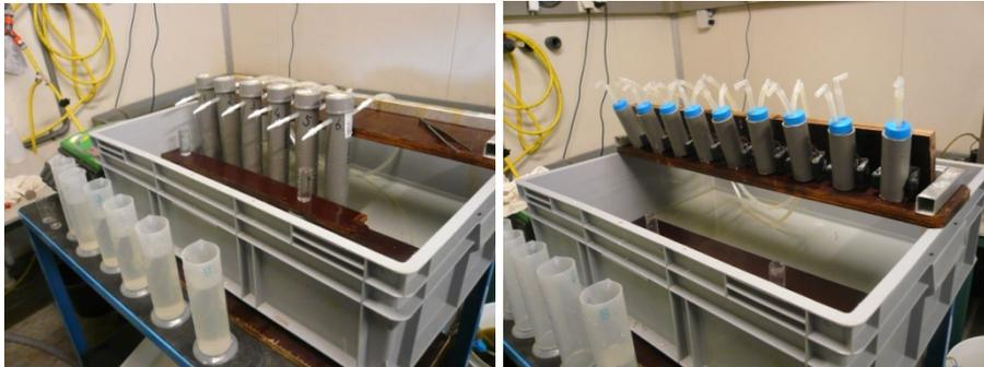
Figure 1. Filtration setup, left for the small clams, right for the big clams.
