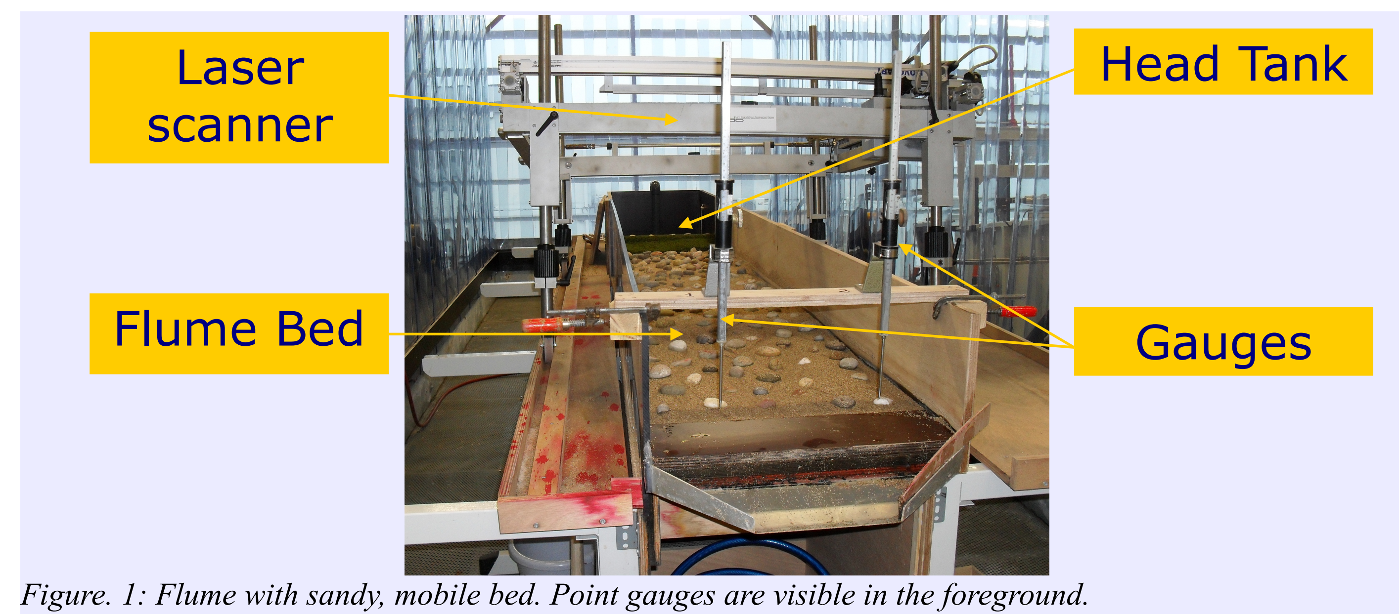
Figure 1: Flume with sandy, mobile bed. Point gauges are visible in the foreground.
