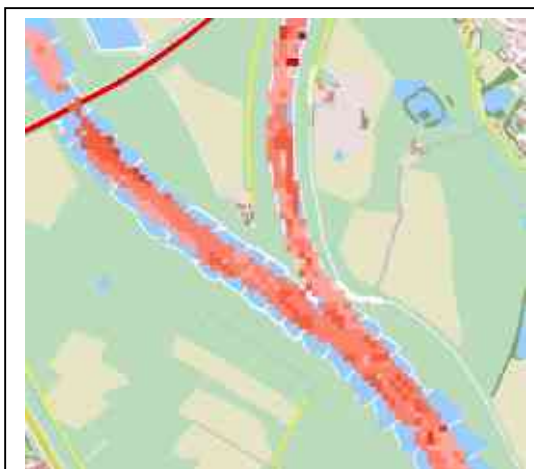
Figure 3a. The calculated Shields parameter ( \theta ) for two realizations (a and b), only minor differences can be seen, leading to no differences in whether or not the sediment is transported in this example ( \theta_{cr}=0.06 ; threshold of motion).
