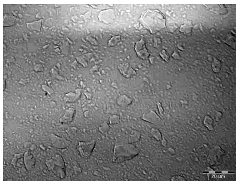
Figure 2.2 Optical microscopic image of microgel particles dispersed in water (same DO30% microgel sample indicated in figure 2.1), scale bar shown in graph is 20 \mu\text{m} .
