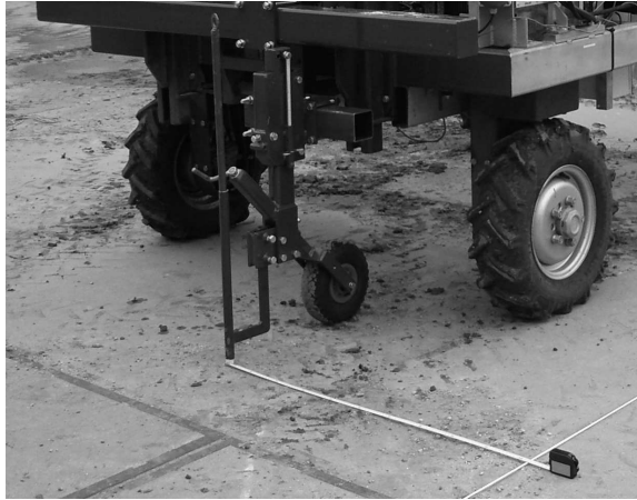
Fig. 7. Chalk holder attached to the robot. To the right of the the robot the rope indicating the path is visible
