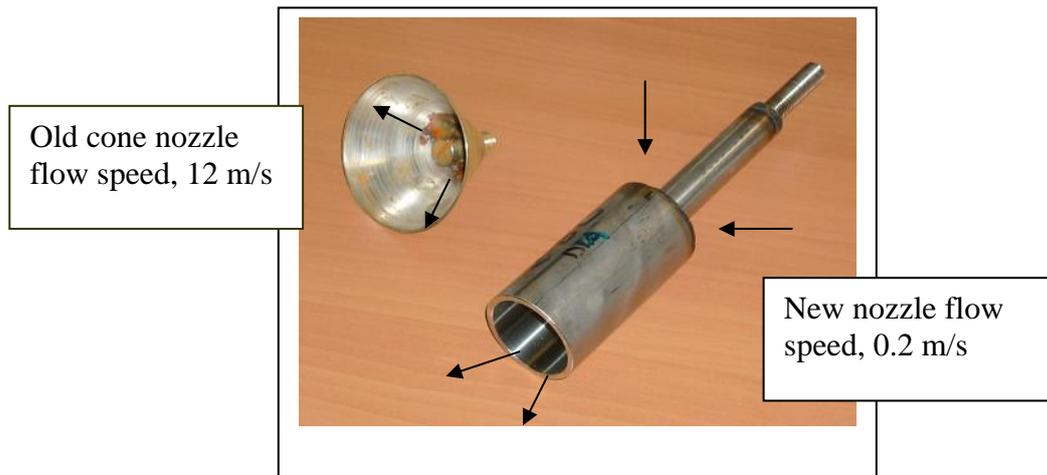
*Nozzle flow speed of the old and new nozzles*
