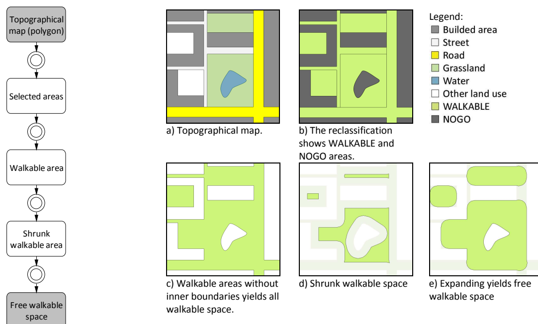
Figure 4) In this figure the process of deriving free walkable space is shown. First the scheme (left) subsequently a visualization. The process starts of with a topographical map (a), next a reclassification (b), then the boundaries are removed (c), subsequently the areas are shrunk (d) and finally its proportions are restored (e). Note that roads are included at a later stage.
